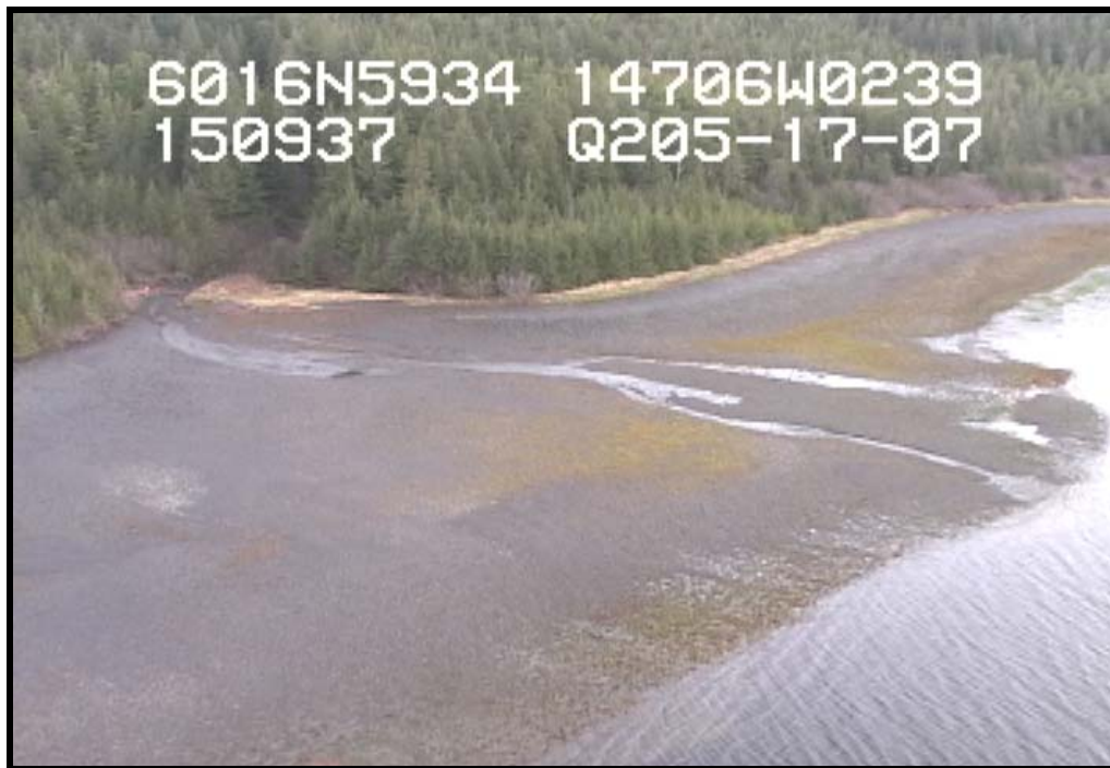
Figure 1.4. Example of a frame capture from video imagery in Zaikof Bay, northern Montague Island, Prince William Sound. Note GPS location, time code, and date burned on imagery, information which is also recorded in the navigational trackline.
