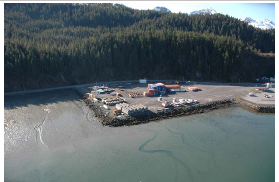
Forms As (seawall) composed of Material Ar (riprap), BC Class 32 (man-made) Cordova (Unit 02/04/7005) PWS07_MM_10417.jpg
