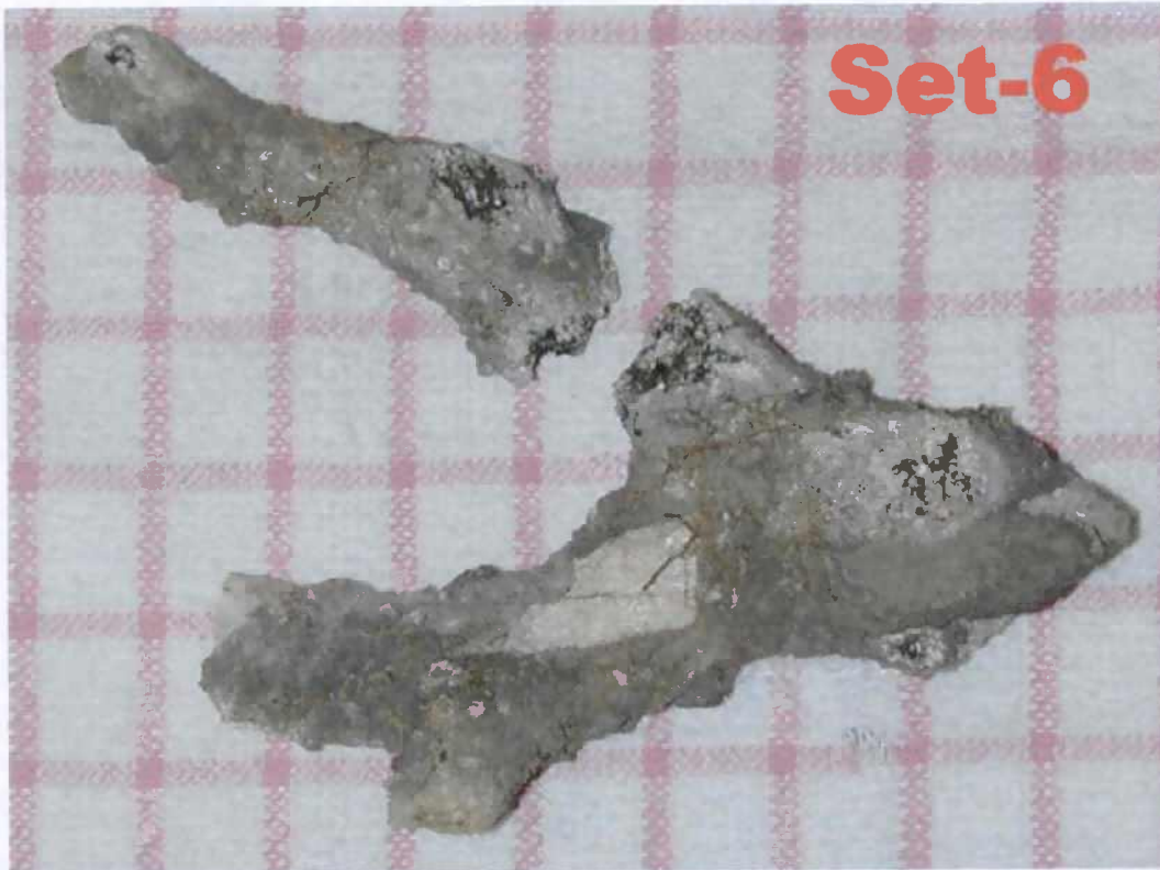
Figure 3. Sample of fulgurite for sale on internet website, showing branching texture of bubbled silica glass.
