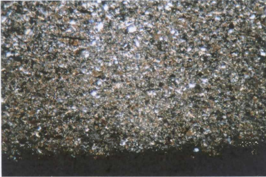
Figure 9. Lowest layer of shale immediate roof exposed at mine roof horizon, showing angular quartz grains (bright white) scattered in a matrix of very fine-grained lathes of muscovite (rectangular, brightly colored yellow/pink/blue). Brown represents patchy iron staining. Field of view 2.4 mm at 40X, taken under crossed polars.
