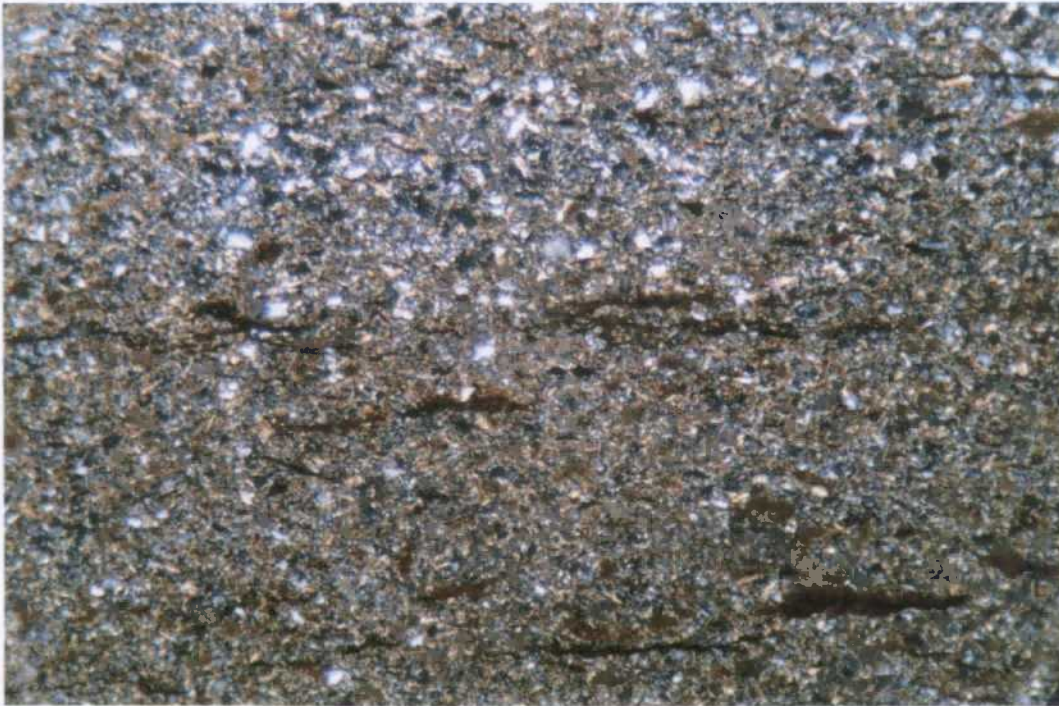
Figure 18. Very regular, continuous bedding contact between lower, fine-grained lamination characterized by scattered, angular quartz grains (bright white) in a very fine-grained matrix of muscovite (speckled yellow/pink), grading upward into lamination with abundant, angular quartz grains. Some quartz grains touch along tangential contacts, while most are isolated by surrounding muscovite. Discontinuous stringers of iron hydroxide (black to very dark brown), which may represent diagenetic alteration of original biotite flakes, are aligned parallel to define bedding. Field of view 2.4 mm at 40X, taken under crossed polars.
