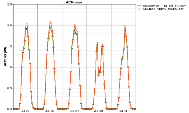
Fig. 3: Comparison of hourly results from the Sandia model (green-symbols) and CEC model (red-no symbols)
