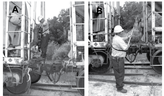
Figure 2. Setting brakes (a) after mounting railcar, (b) using brake stick.
