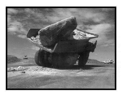
Excessive overloading and/or load bias beyond design parameters may lead to the likely failure of critical components and instability which may seriously jeopardize safety.
