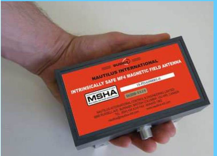
MF4 Magnetic Field Antenna located on CM Weight: 1.8 Lbs
