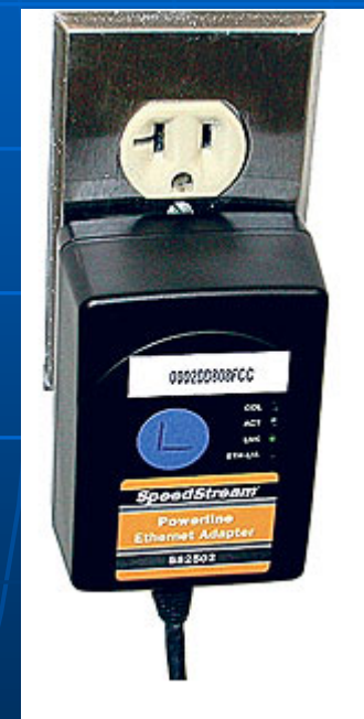
HomePlug Modem can turn an electrical outlet into an Internet connection.
