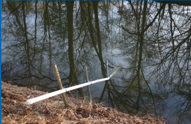
Continuous recording of stage and water temperature.
