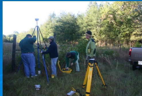
RTK GPS to convert stage to actual elevations
