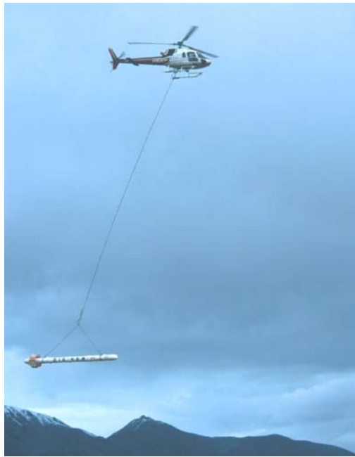
Figure 159 . Helicopter conductivity measuring system. (Fugro Airborne Surveys and John Holland, ERA Helicopters)
