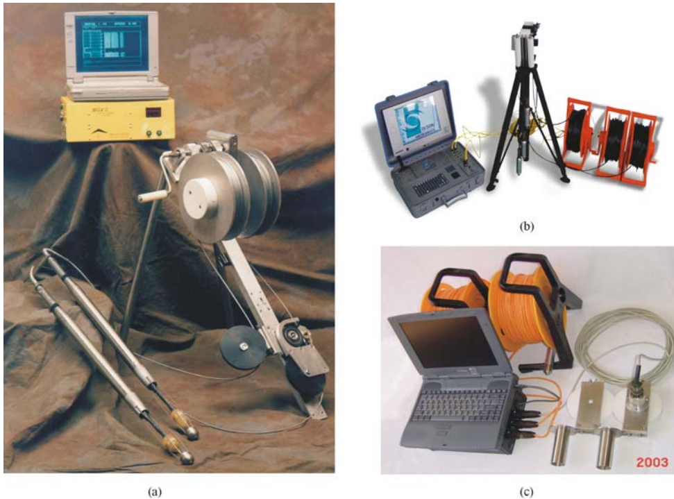
Figure 18. Crosshole Sonic Logging instruments. (a) InfraSeis, Inc., (b) Olson Instruments, Inc., and (c) GeoSciences Testing and Research, Inc.
