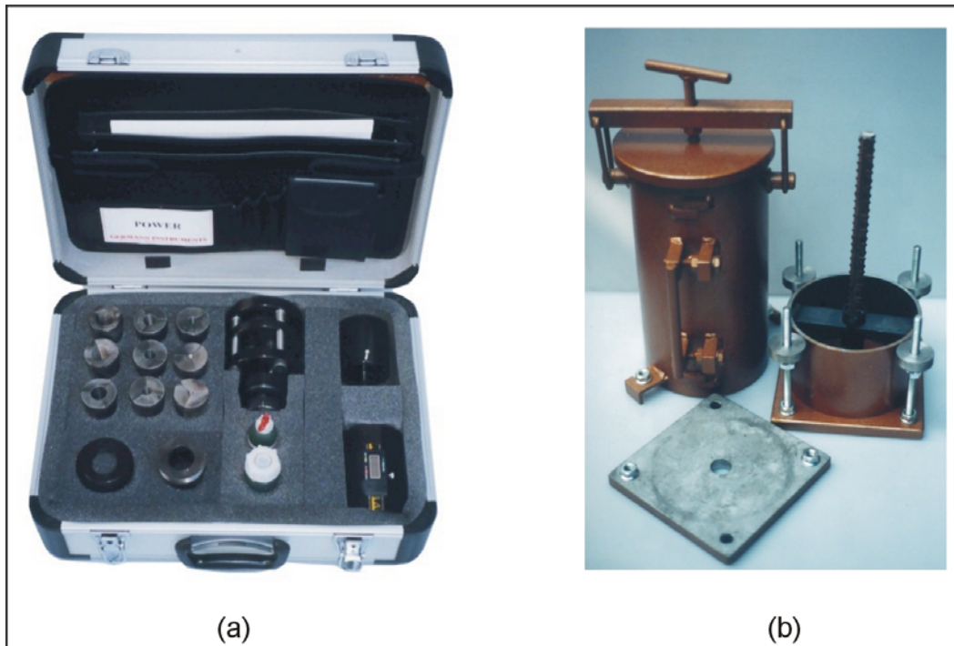
Figure 38. Power equipment to test rebar bonding: (a) Preparation Kit, and (b) Power equipment. (Germann Instruments)
