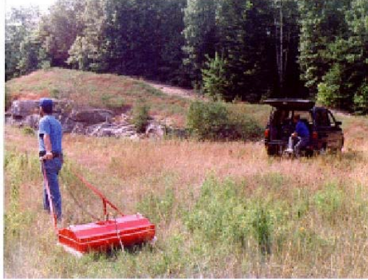
Figure 113. Ground Penetrating Radar antenna (100 MHz) used in a survey. (MALA GeoScience USA, Inc.)
