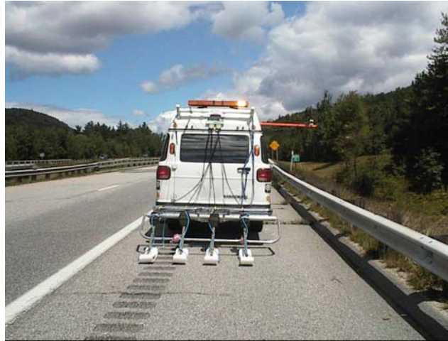
Figure 73. Ground Penetrating Radar Method Two: low speed, high-resolution using four 1.5 GHz antennas spaced equal distance apart. (Geophysical Survey Systems, Inc.)
