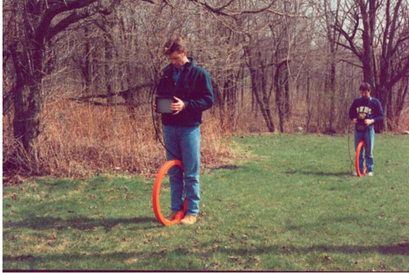
Figure 197. The EM34 being used in horizontal dipole mode. (Geonics, Ltd.)
