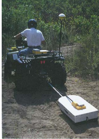
Figure 139. A 250 MHz antenna being used in a field survey. (MALA GeoSciences, Inc.)
