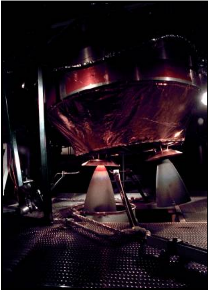
Cassini – Saturn Orbit Insertion Engine Glows during 3-h 20-min Continuous Firing
