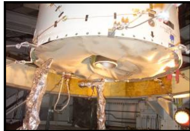
Minuteman Qualification Firing inside Vacuum Test Cell
