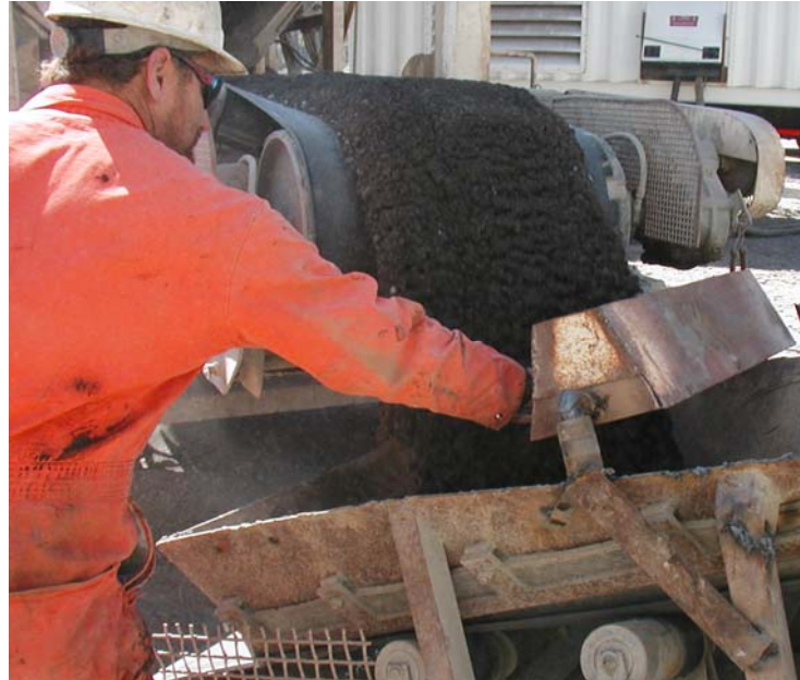
Exhibit 3-7 Sampling Device Cutting Across Flowing Stream
