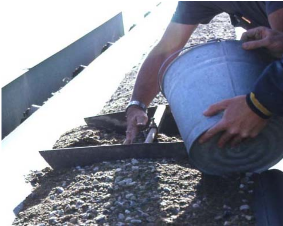
Exhibit 3-8 Sampling from Conveyor Belt
