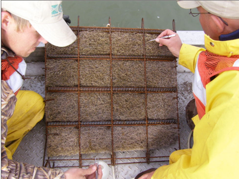
Figure E5. Mats used to sample eggs on coarse substrate deposits.
