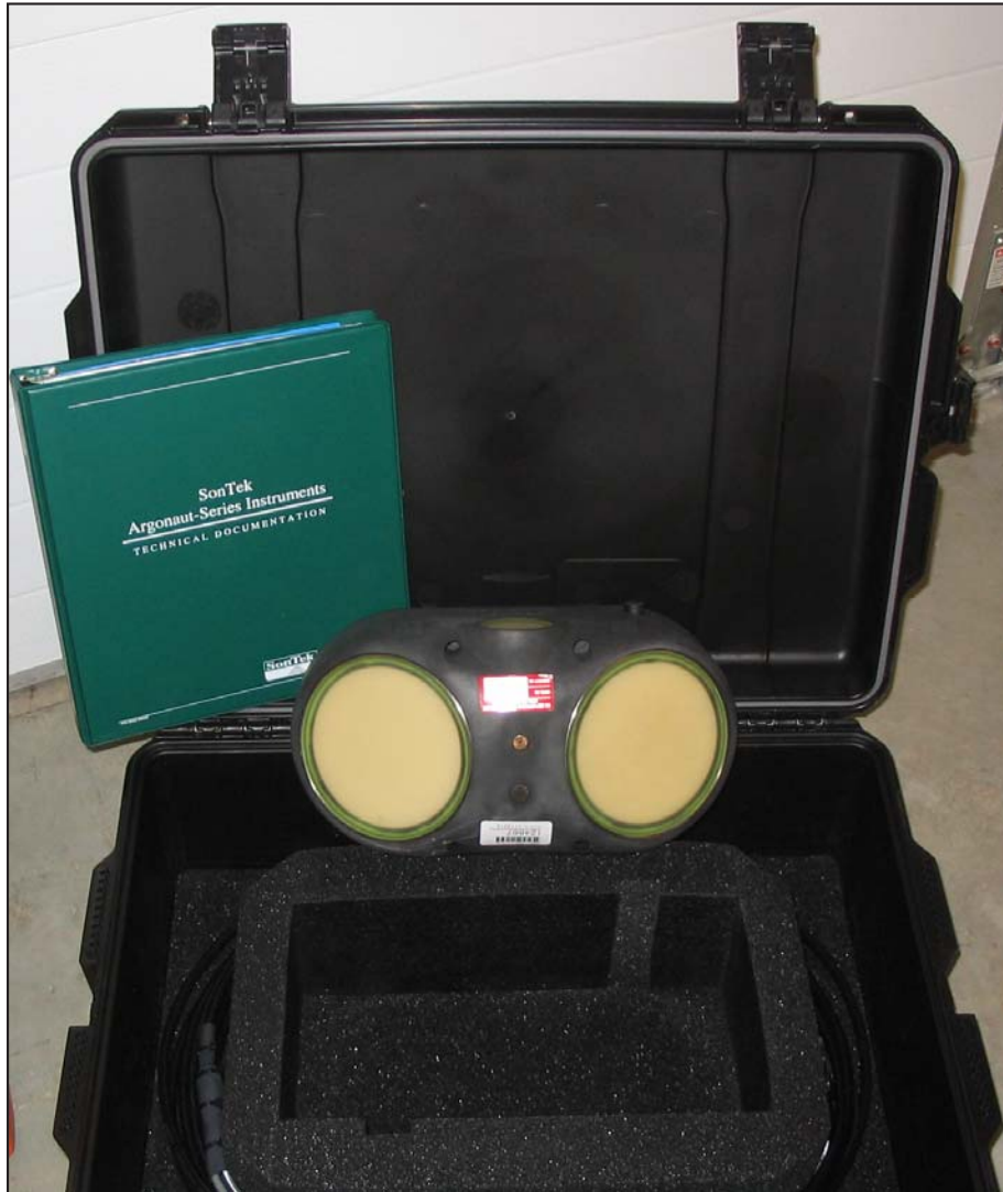
Figure F2. SonTek acoustic Doppler velocity meter (Sontek/YSI incorporated, San Diego, Calif).
