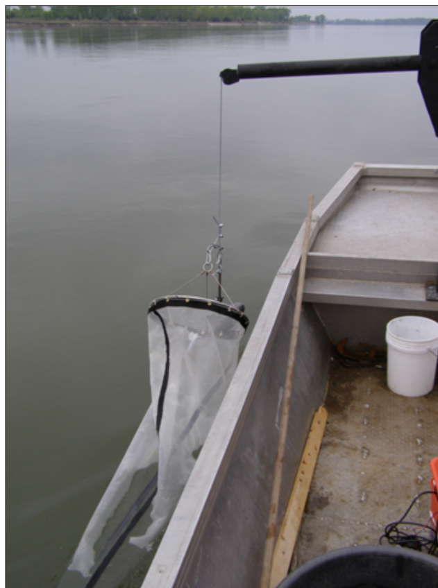
Figure E6. Lcthyoplankton net with 750-µm mesh attached to a 75-lb (34 kg) Columbus-style sounding weight used to sample drifting larval fishes.
