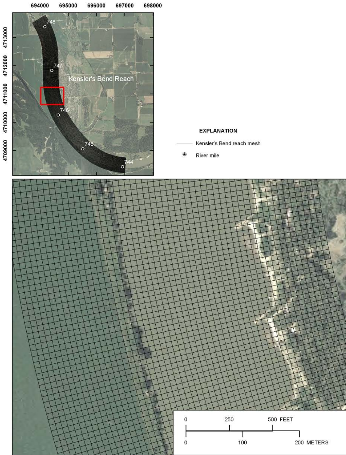
Figure D26. Multi-Dimensional Surface Water Modeling System mesh at Kensler's Bend. Mesh was created by using elevation data from the bathymetric and terrestrial surveys.
