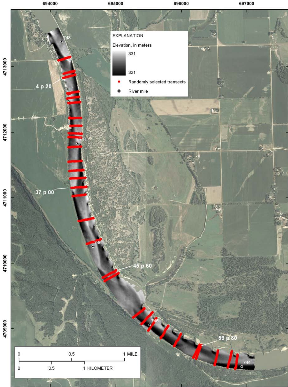
Figure D34. Randomly selected transects at Kensler’s Bend reach. The randomized sample was used to provide unbiased estimates of areas of the reach affected by flow and transport processes. Transects were surveyed four separate times throughout the year (2006) at various discharges. Transects with identification are for referencing in other figures.
