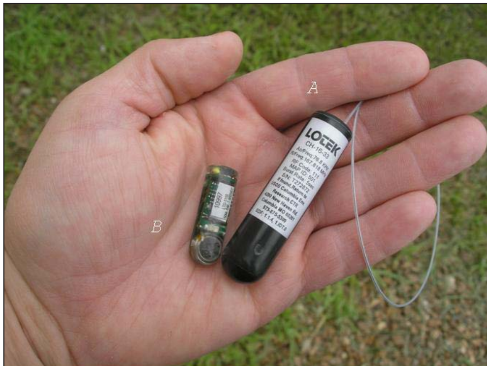
Figure B2. Lotek (Lotek Wireless Inc., Newmarket, Ontario, Canada) combined acoustic/radio transmitting (CART) tag implanted in shovelnose sturgeon in 2006 (A) and data storage tag (DST) implanted in all sturgeon in 2005 and 2006 (B). Transmitters implanted in 2005 were acoustic-only tags of similar size but lacking the external antenna.
