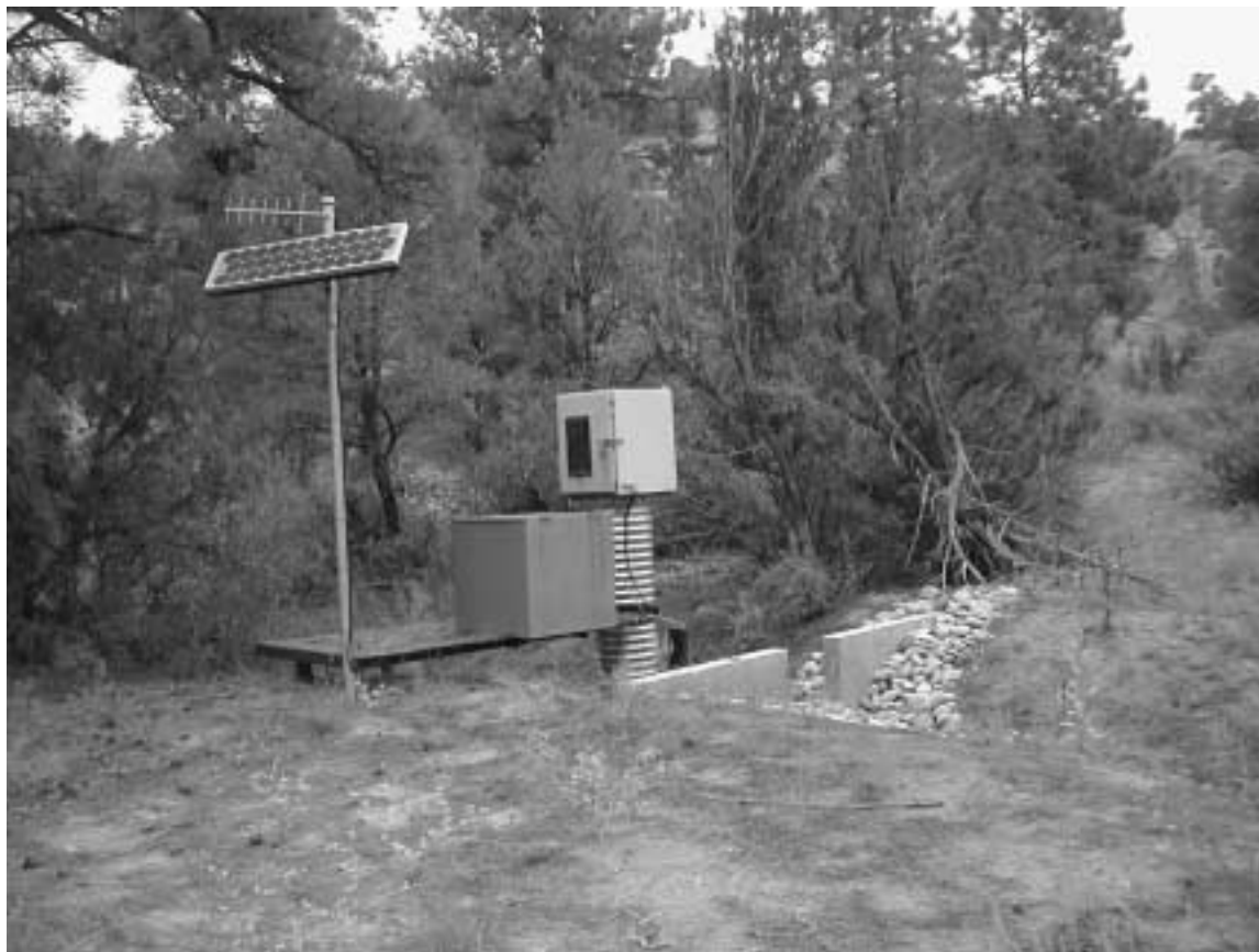
Figure 3. Typical automated storm water sampler.
