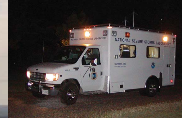
NSSL mobile lab/mobile field command that is equipped to receive data from aircraft, lightning mapping arrays and ground-based radar and balloons.
