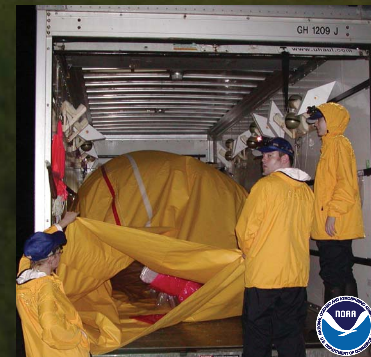
(Right) Crew members in a truck configured as a mobile inflation shelter inflate a balloon and check out instruments for the next flight. Inflating a balloon in its launch tube allows it to survive handling and launch in strong winds.
