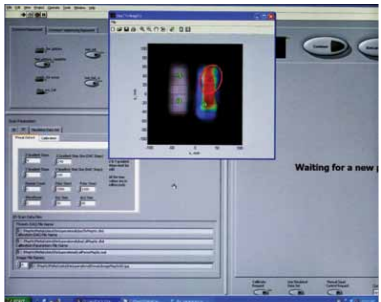
The screen of the MagViz unit displays each tray of liquid or gel items, with the target materials highlighted by color according to potential risk.
