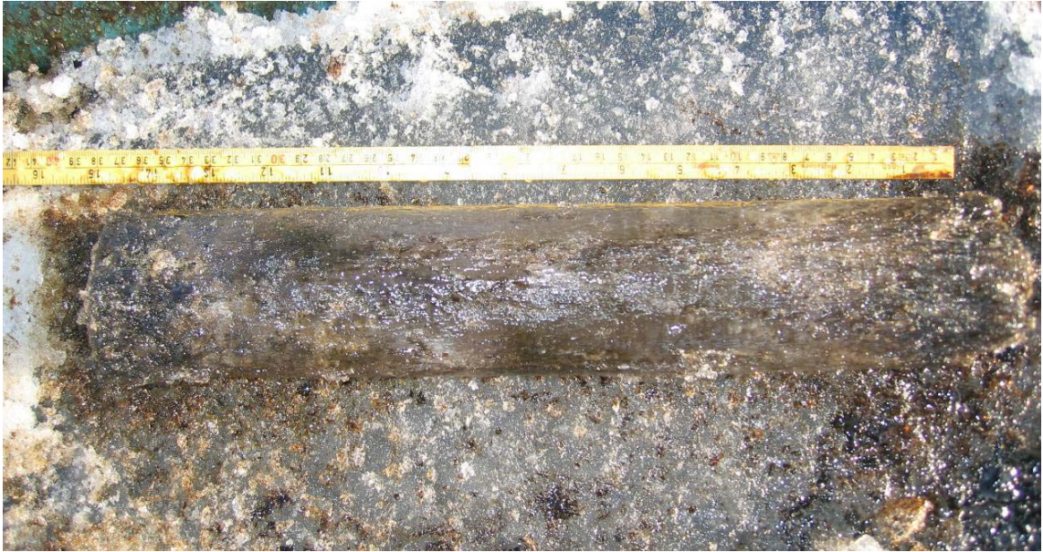
Figure 4: One of the ice cores taken inside the skirt on May 04, 2006. Considerable amount of oil can be seen in evenly distributed in the brine channels as small droplets. Very little oil is present under the ice.
