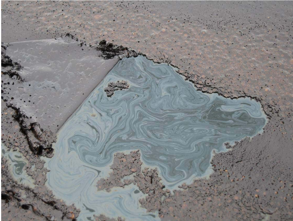
Figure 7: The burning residue of the Statford crude is solid and very easy to recover by simple mechanical means.
