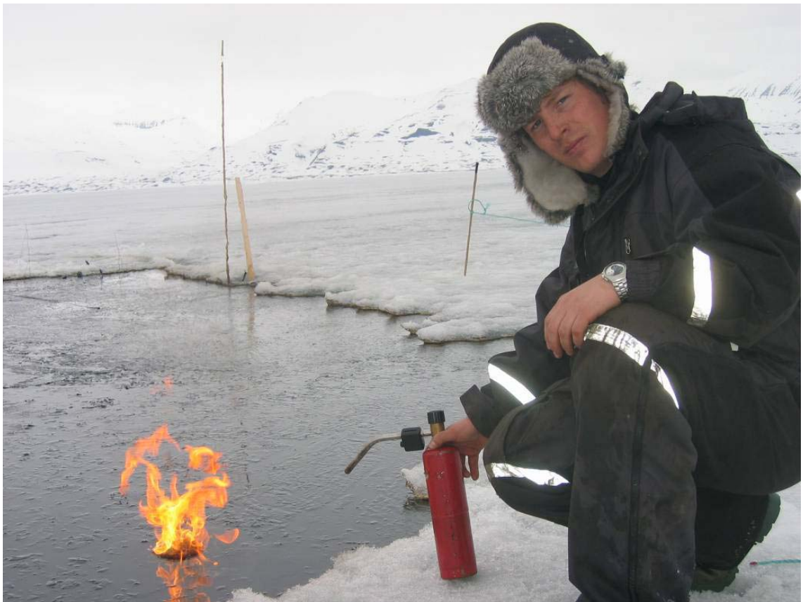
Figure 5: Ignition of the surface oil on May 30. using a 250 ml of gellified gasoline and a small propane torch by the MSc student Roger Daniloff (NTNU/UNIS).
