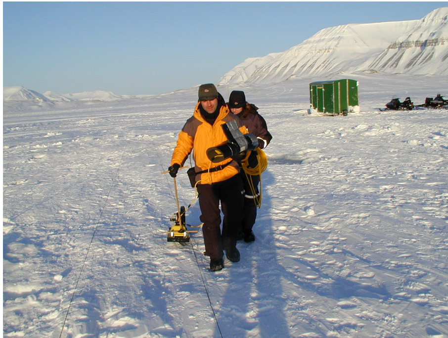
Figure 3.3: Ground based GPR data acquisition along established gridlines with the 500 MHz system.
