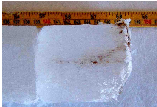
Picture 11: Close-up of oil in brine channels within the lower 8 cm section of a 23 cm core taken from Location 3 inside the oiled area on March 29 (Figure 3.4)
