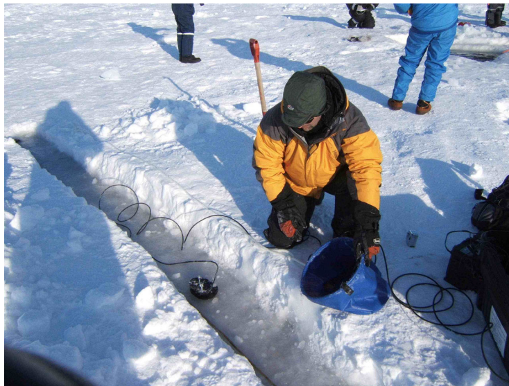
Picture 27: Acoustics profile with sonar transducer on wetted ice surface in test trench extending from outside to inside oil skirt
