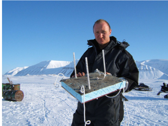
Picture 8: SINTEF prototype under-ice oil thickness sampler used to measure oil film thickness under ice, May 26.2006.
