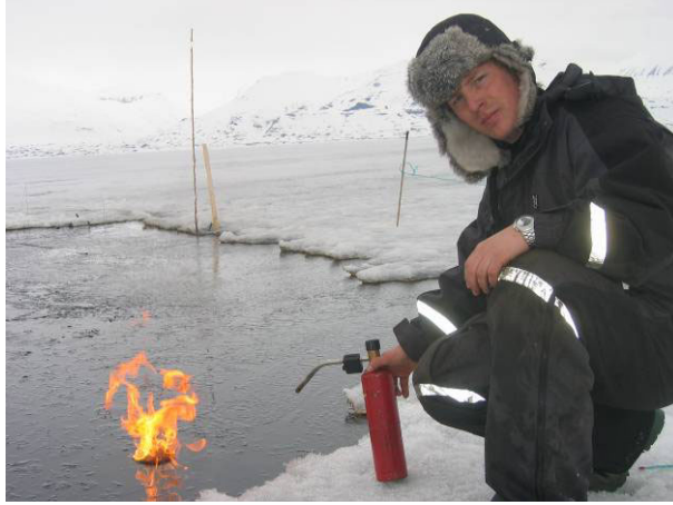
Picture 16: Ignition of oil with handheld igniter (a slab of gelled n-hexane on the oil and butane torch). May 30, 2006.
