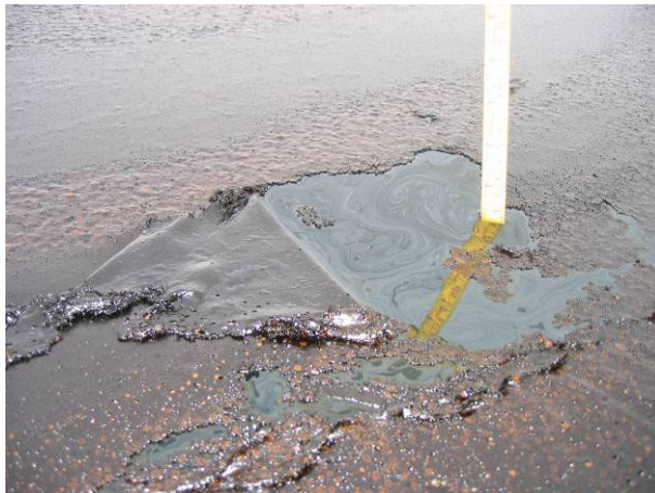
Picture 19: In-situ residue after 2 hours of cooling. Semi-solid, thickness 1 mm. May 30, 2006
