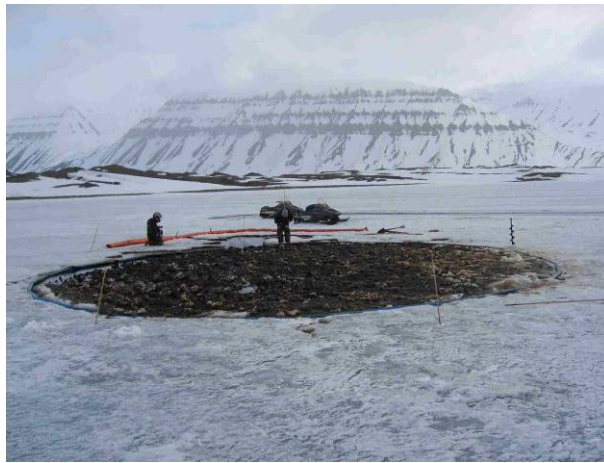
Picture 14: Oil in the melt pool on the ice, May 10, 2006.
