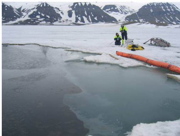
Picture 15: Oil in the melt pool on the ice, May 30, 2006.
