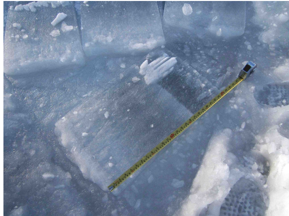
Picture 6: Ice block total thickness 62 cm floating on its side in the dive hole showing transitions in ice structure from random orientation to columnar at ~15 cm and to clear slower growing ice with less air intrusions) at a depth of 44 cm
