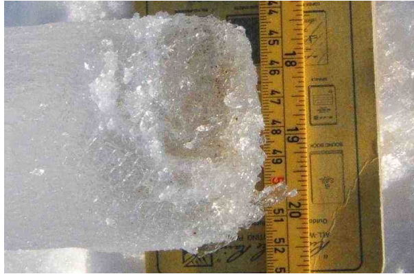
Picture 10: Close-up showing small oil drops (0.2 to 1 mm) in the bottom 2.5 cm of a core taken outside the oil skirt on March 29, 48 hours post-spill (Ref.3 location in Figure 3.4)
