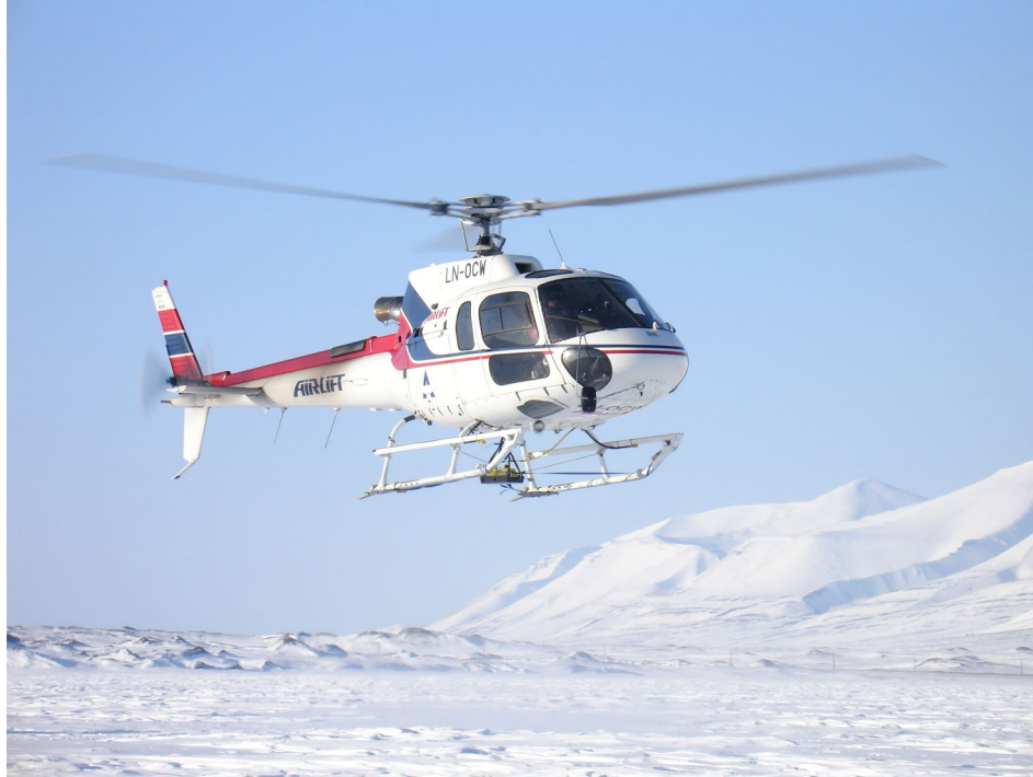
Figure 4.7: The airborne system configured with the 500 MHz antennas, which are visible between the skids. The antennas are connected via coaxial cables to the recording system within the cabin.
