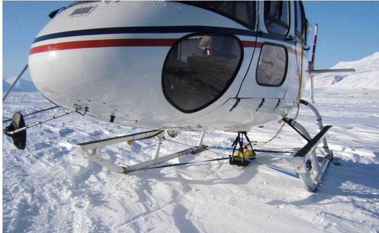
Picture 25: Radar antenna mounted between the skids on AS350 of Airlift AS
