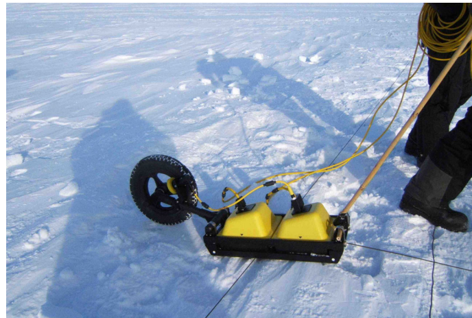
Picture 22: Radar traverse along survey grid line
