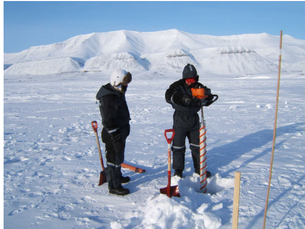
Picture 4: Taking a reference ice core outside the skirted area before the oil release, May 26, 2006
