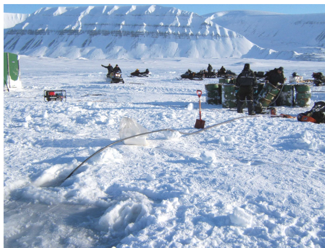
Picture 3: Pumping oil from drums through flexible pipe inserted 1 m inside skirt through a sloped hole drilled 2 m outside, May 27, 2006
