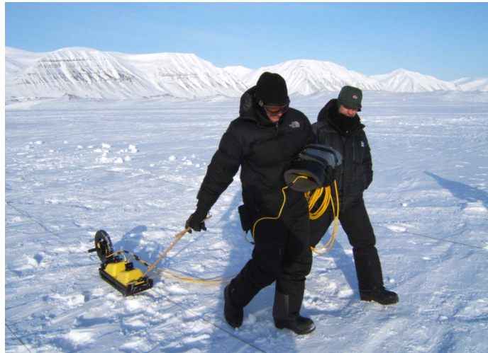
Picture 22: Radar traverse along survey grid line
