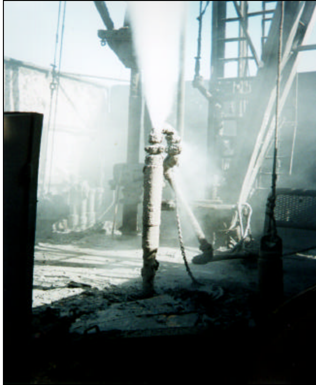
Figure 14– Drill Pipe Blowout
