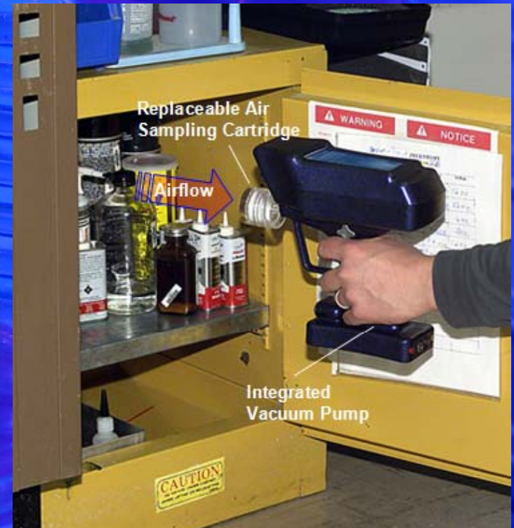
Example of air sampling of a chemical storage cabinet.
