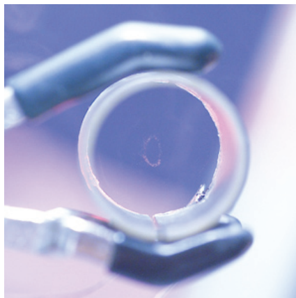
An Aerosonic tube uses acoustic energy to concentrate particulates in an aerosol.
