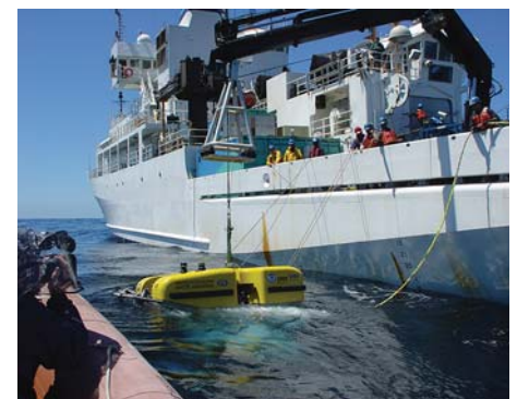
A remotely-operated camera is lowered over the side of the ship.
