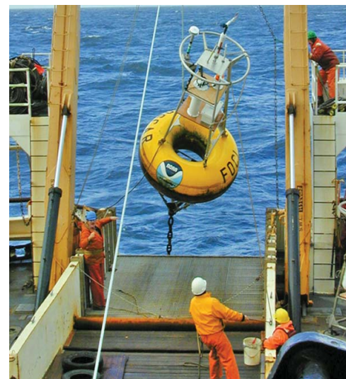
The ship deploys a Fisheries-Oceanography Coordinated Investigations project buoy
