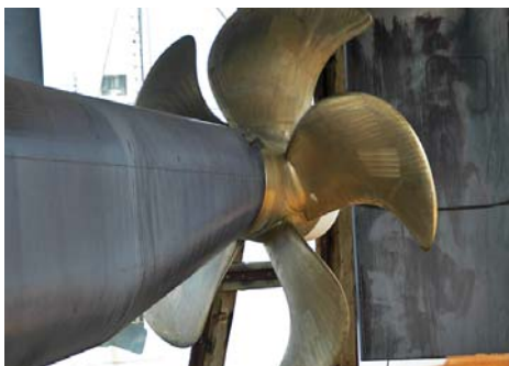
The propeller is specially designed to reduce noise levels, which will enhance NOAA's ability to assess fish stocks.
