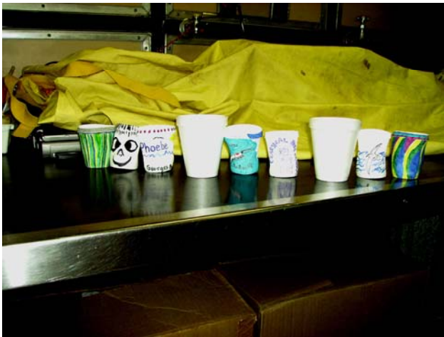
The results of what happened to the cups at a depth of 200 meters. The white cups are the original size.
