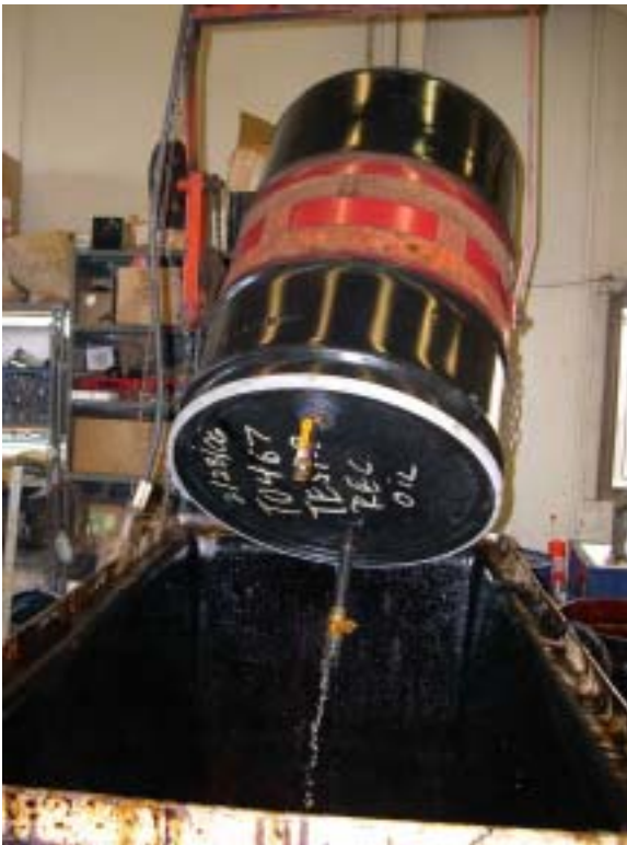
Figure 6. Drum Decanting Method. (Air inlet tube to bottom of drum is placed in drum bung. Water is decanted from drum vent when drum is inverted.)
