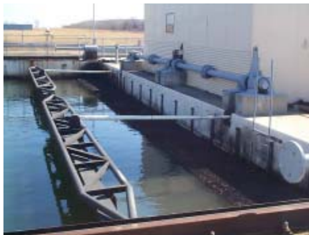
Figure 2. Ohmsett Tank Wave Paddle System
