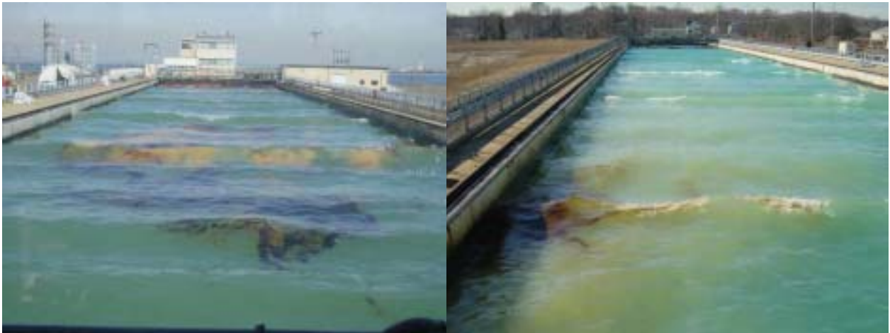
Figure 1. Ohmsett Test Tank with Oil Containment Boom (looking north and then south)
