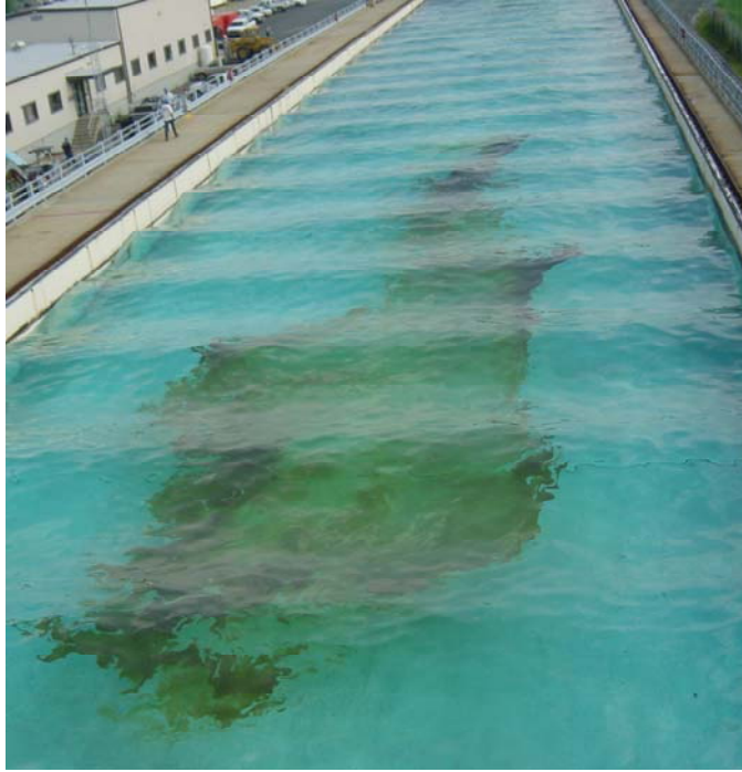
Figure 1 Oil Slick on Non-Breaking Waves
