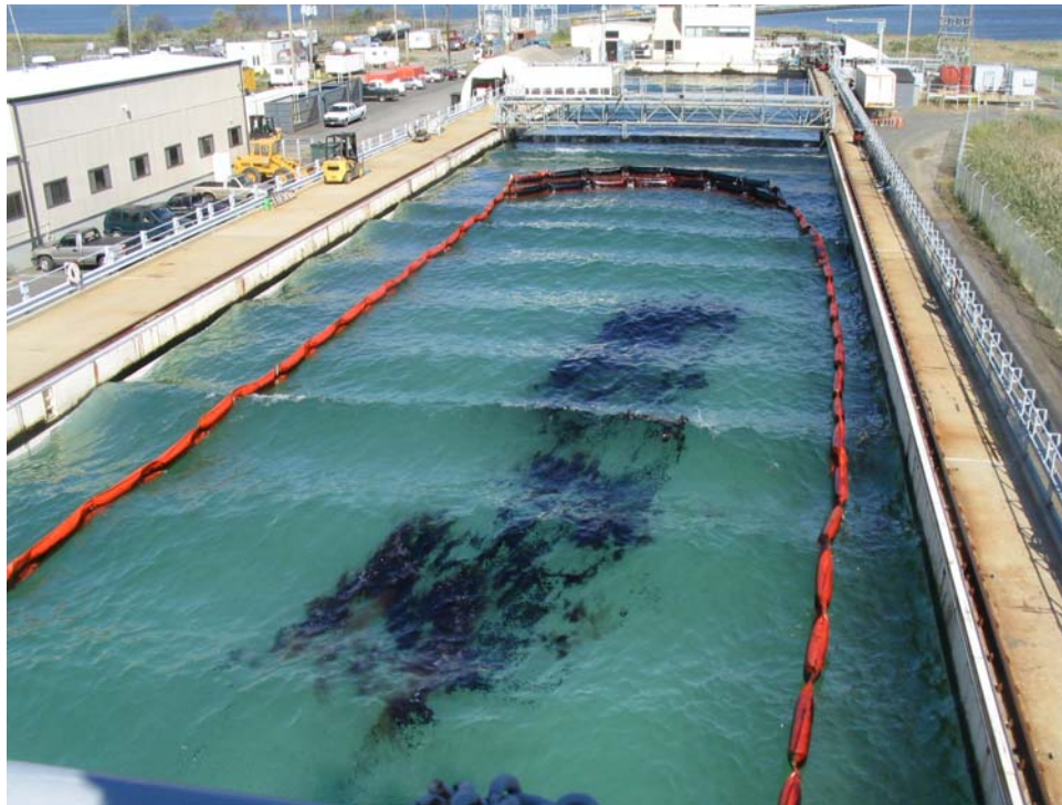
Figure 2 Oil Slick on Non-Breaking Waves (see center of photo).
