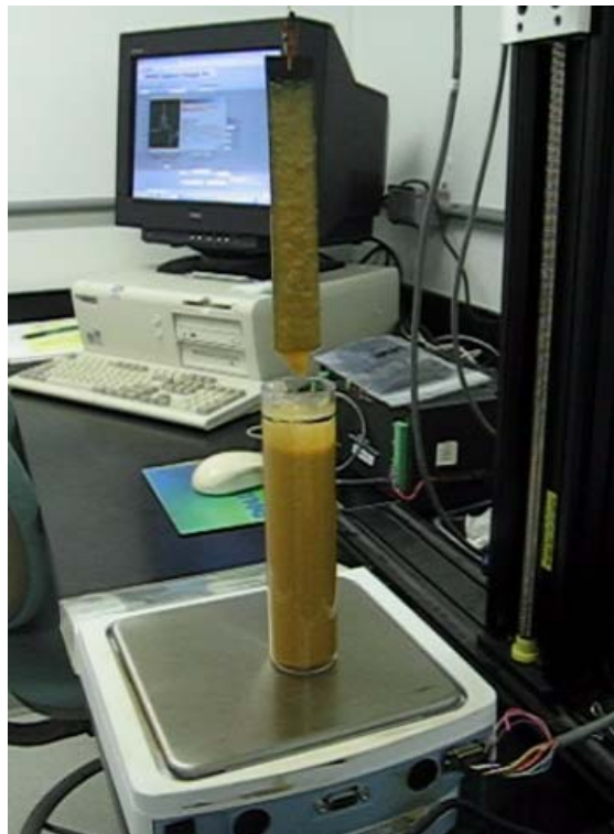
Figure 34. Dip-and-withdraw test for emulsified HydroCal.
