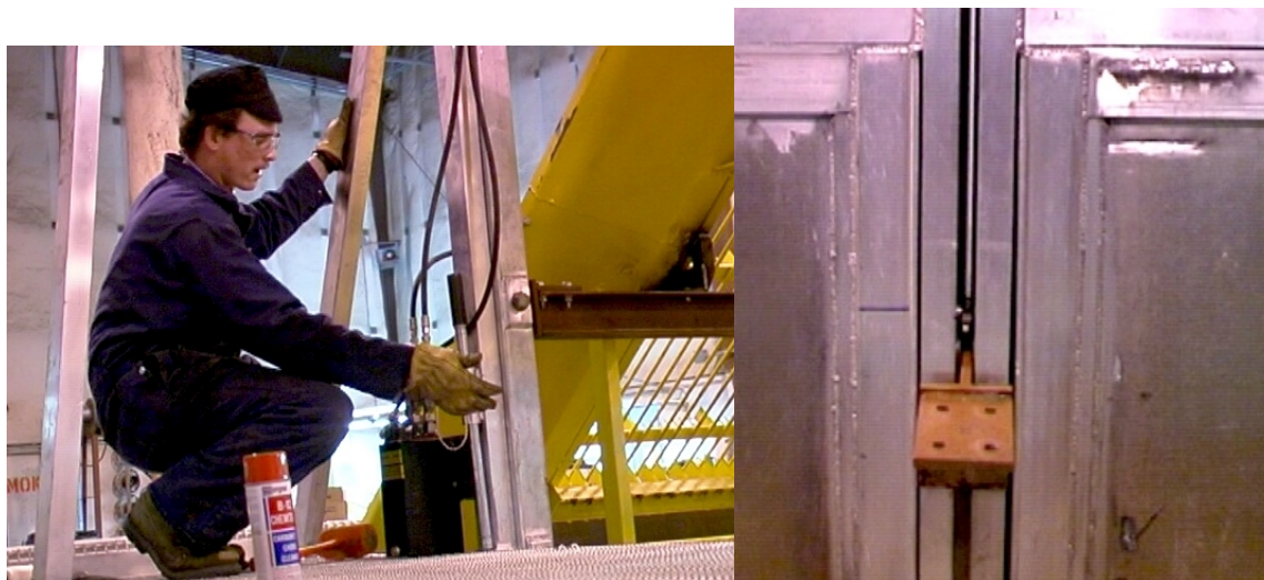
Figure 3.2 Lifting system, handpump (left), ram protected inside post (right).
