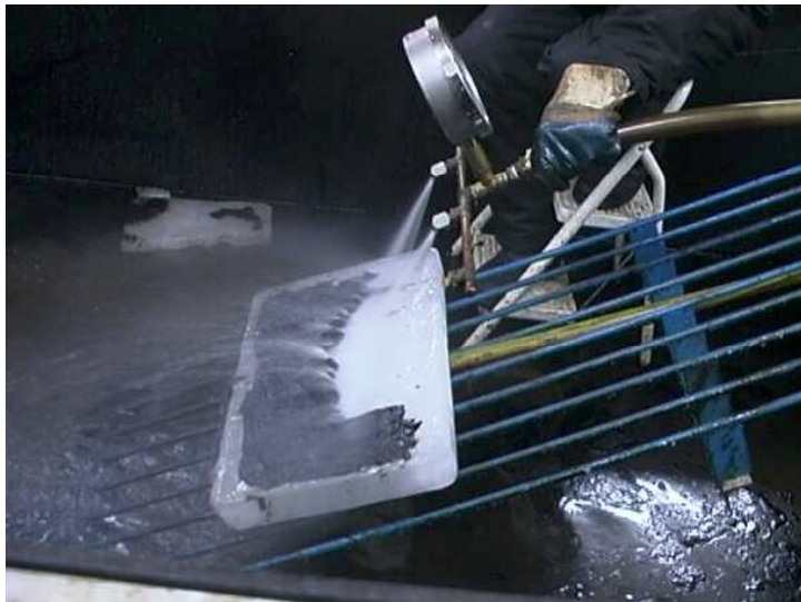
Nozzles with high flowrate, low pressure and low temperature.
