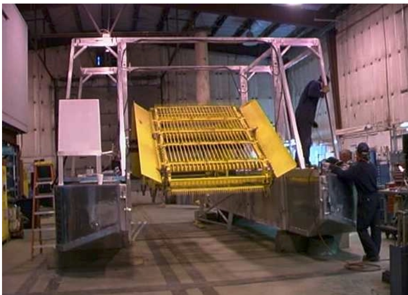
Lifting Grated Belt installed and lifted above seawater line.
