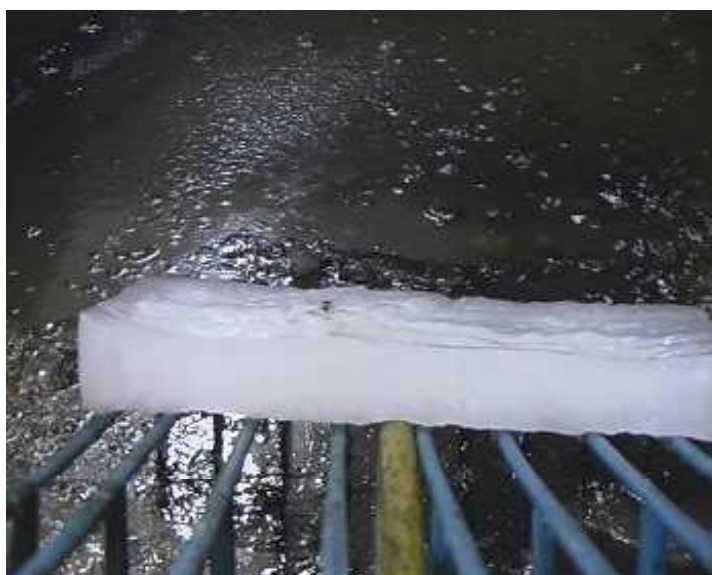
Hot water spray melted a lot of ice before cleaning it.
