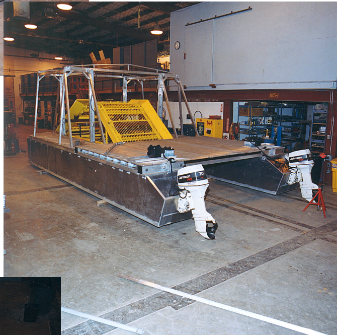
Seen from behind, working deck is ready, outboards installed.
