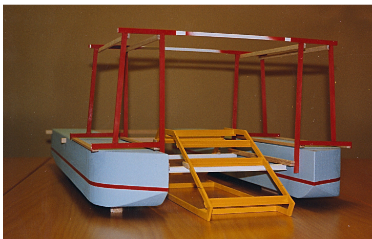
Figure 3.1 Scale model of the work platform and LGB.
