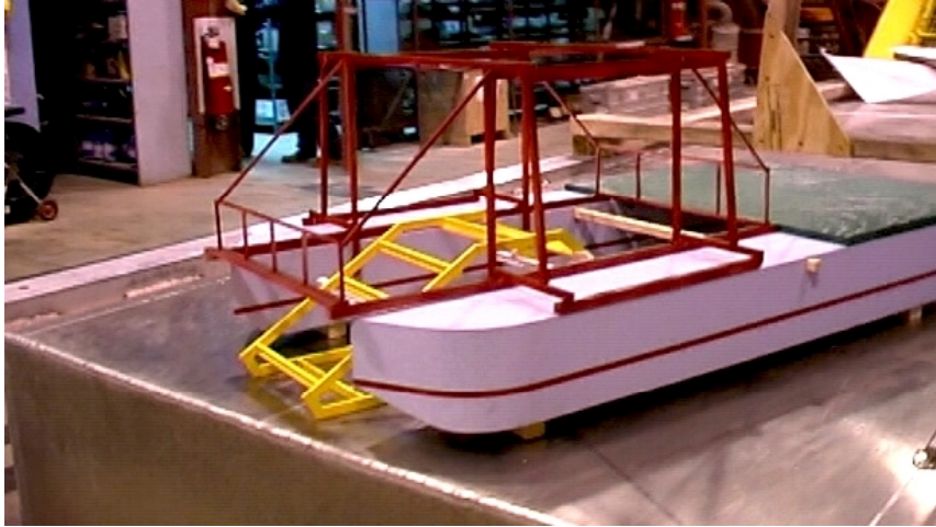
Scale model of work platform with Lifting Grated Belt (yellow), support structure (red) and work deck(green).
