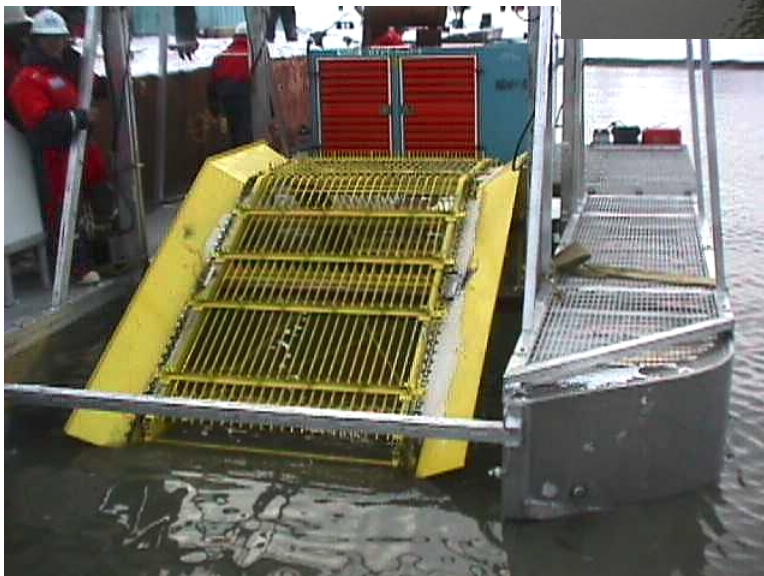
Platform with Lifting Grated belt and a 2 ton hydraulic power pack on deck. The next pictures are with this load.
