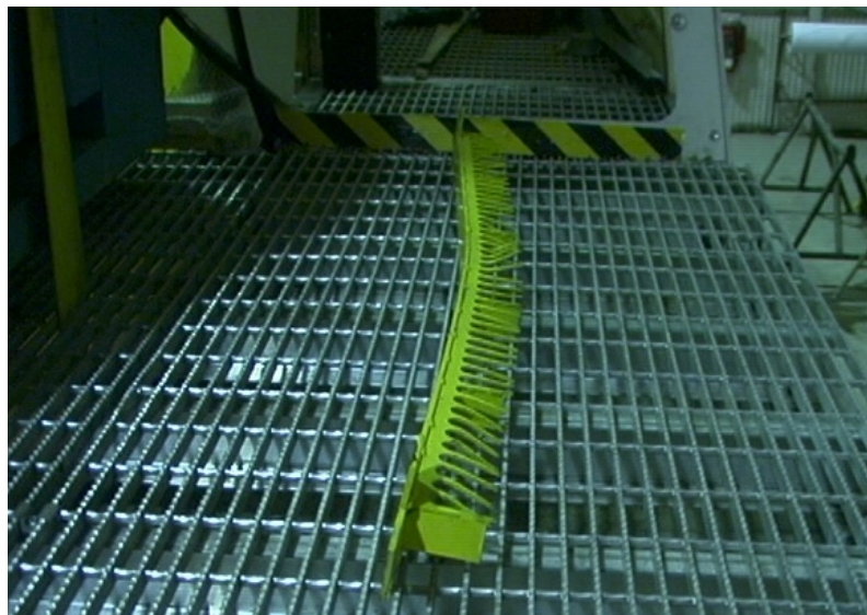
Rakes bent during ice testing.
