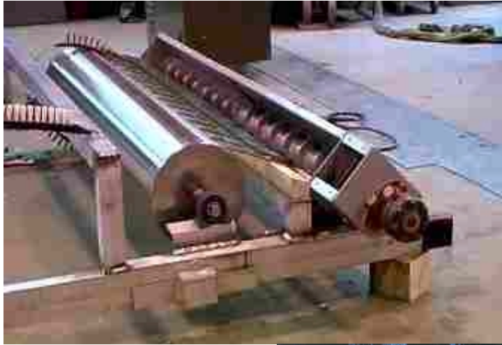
Drum and trough with screw auger under construction.
