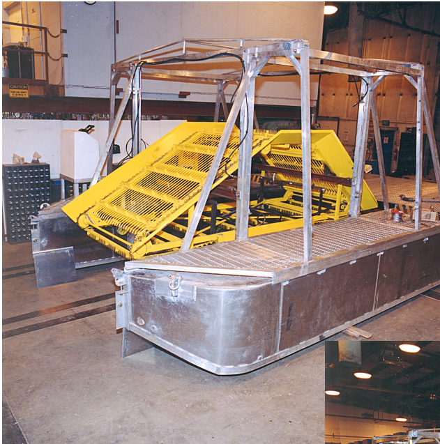
Work platform ready for a float test.
