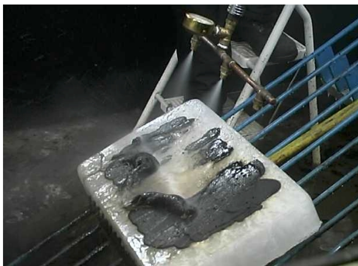
Hot water spray melted a lot of ice before cleaning it.
