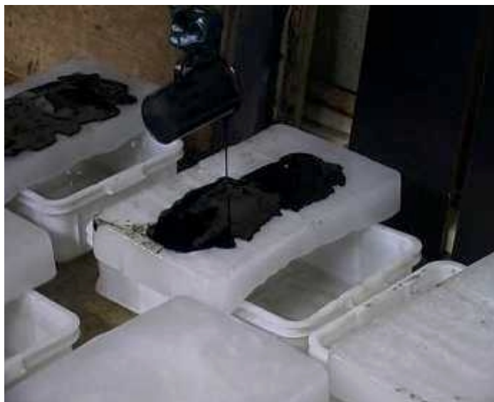
Preparing oil on ice for testing flushing water nozzles.
