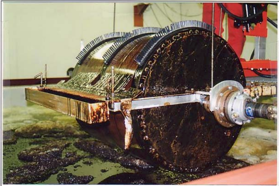
Spiked Drum tested in oil and ice. Three strips of brush 'spikes' measuring 30 cm each are used in one of the initial designs.
