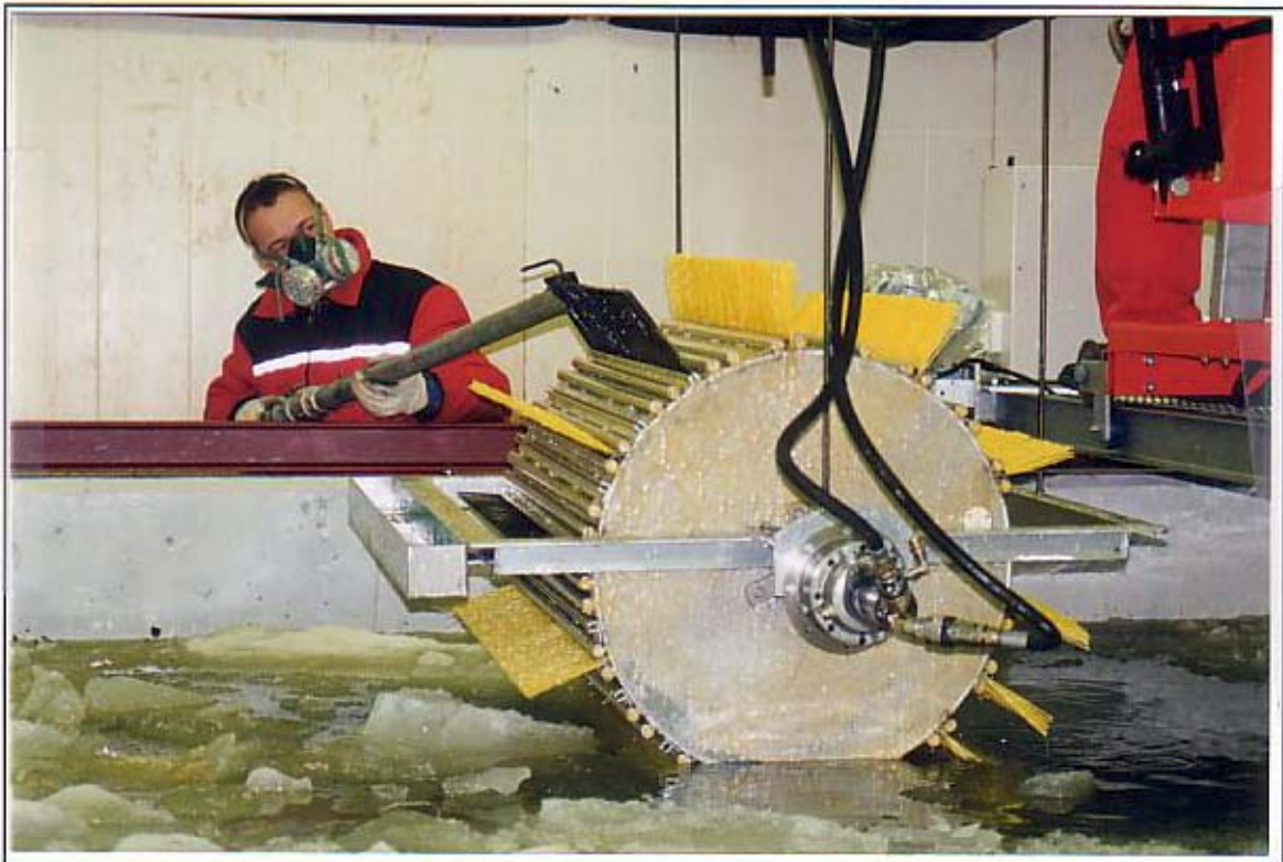
Drum with paddles of different brush types (length, bristle stiffness) being evaluated for its ice deflection capabilities.
