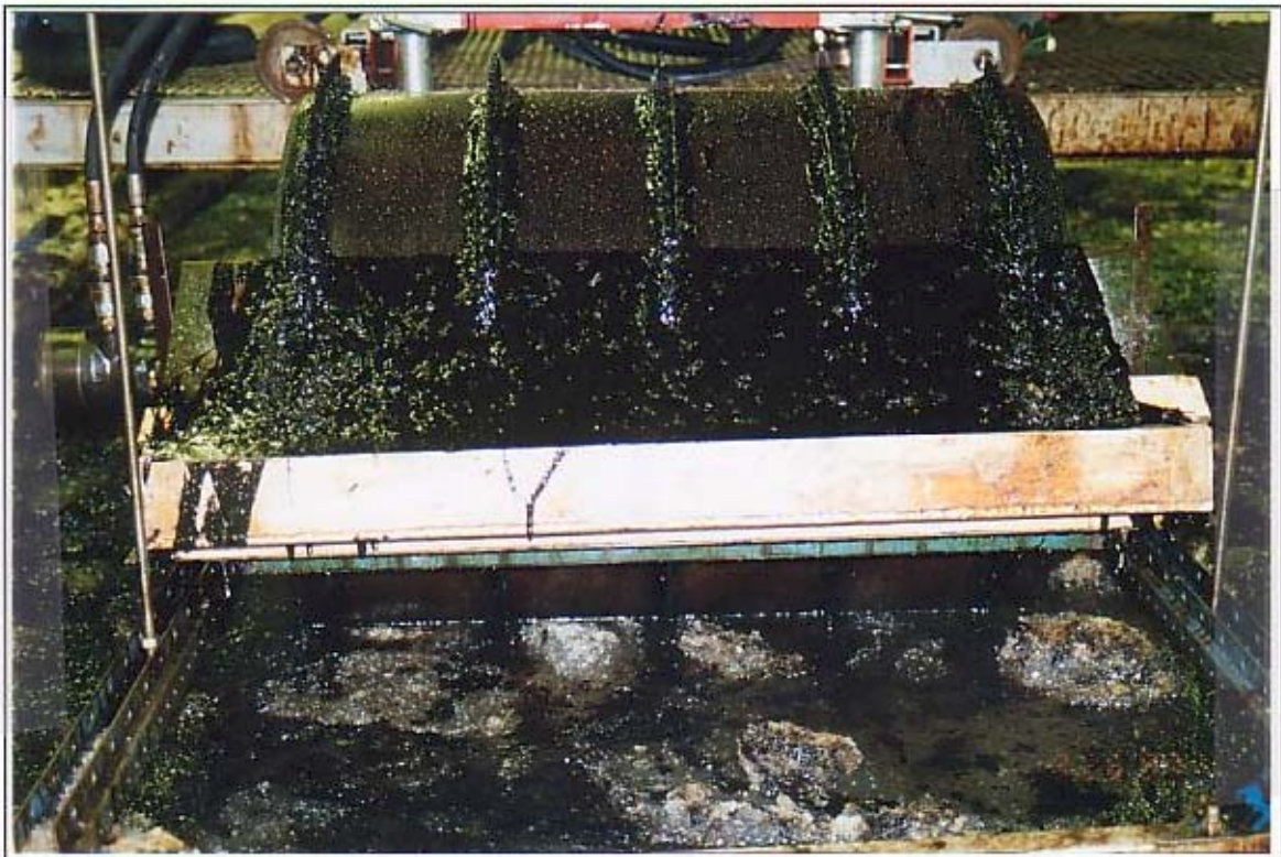
Modified Spiked Drum with five rows of longer strips (50 cm) of spikes and an improved drum scraper
