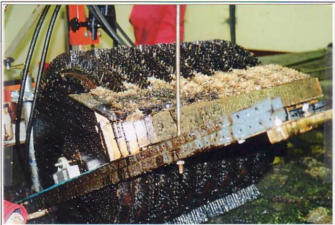
Ringed Brush Drum tested in oil and ice, has a higher slush recovery than the smooth drum, but unlike the latter, can also deflect ice pieces.
