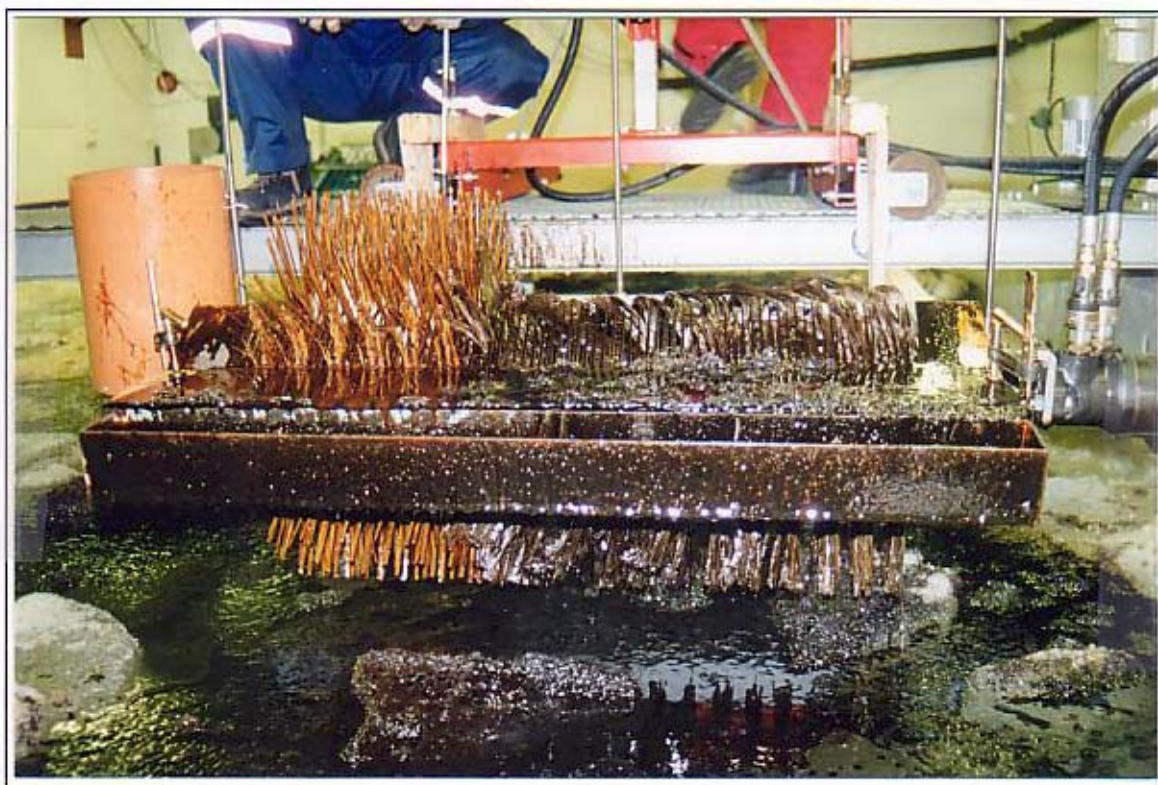
Initial tests with the Brush-Drum concepts. Various bristle types are evaluated for ice deflection and oil recovery performance.
