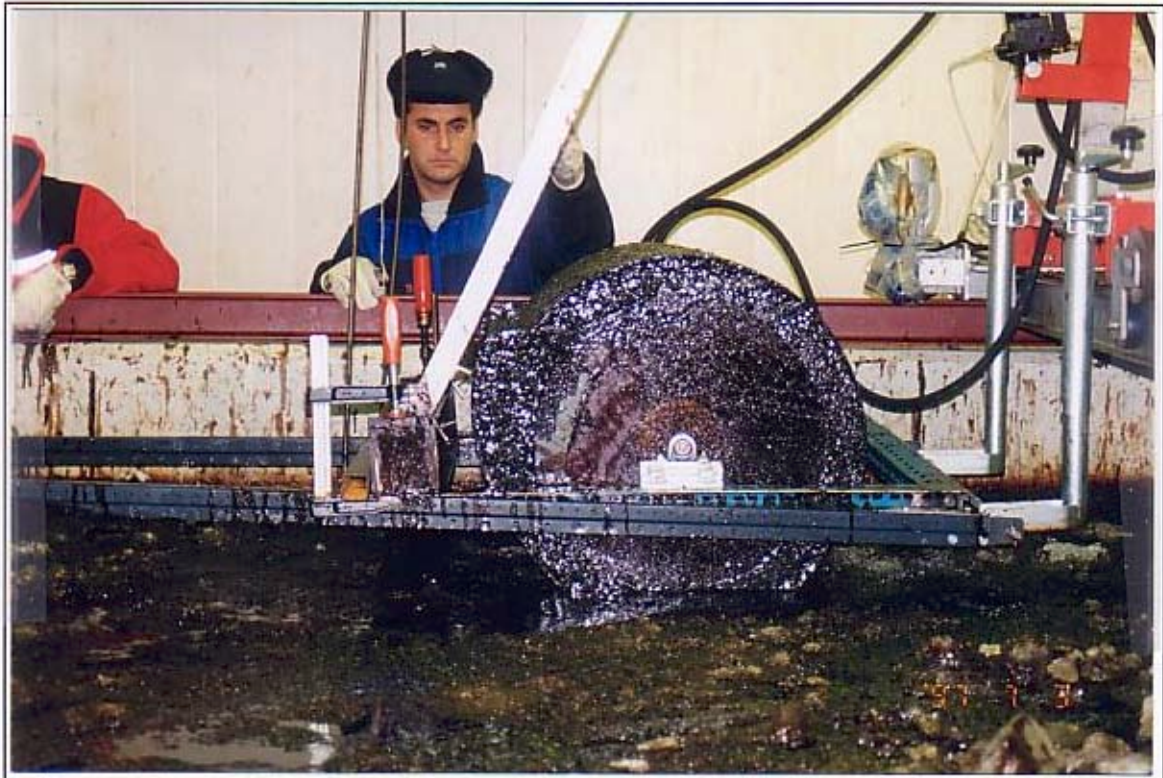
Testing of the paddle-drum concept. A cam lifted away the scraper to allow the paddle to pass. This unit appeared to have a limited ice-processing ability.
