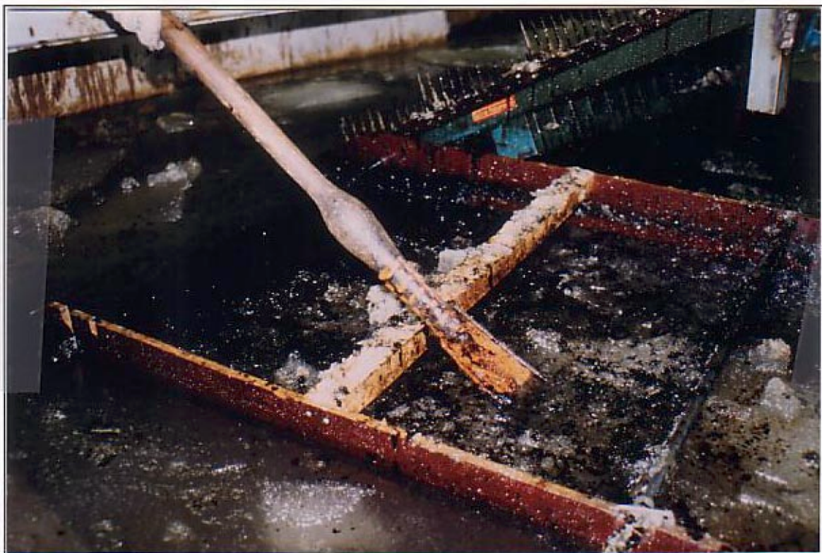
Oil and slush accumulated in the reservoir under the belt. Most of the oil was found on top of the slush layer.
