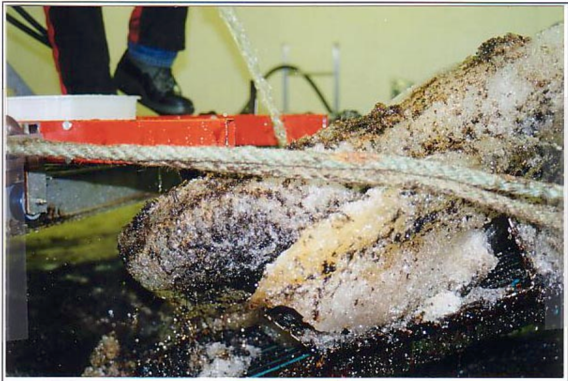
The oil used for testing was flushed relatively easy off the ice.
