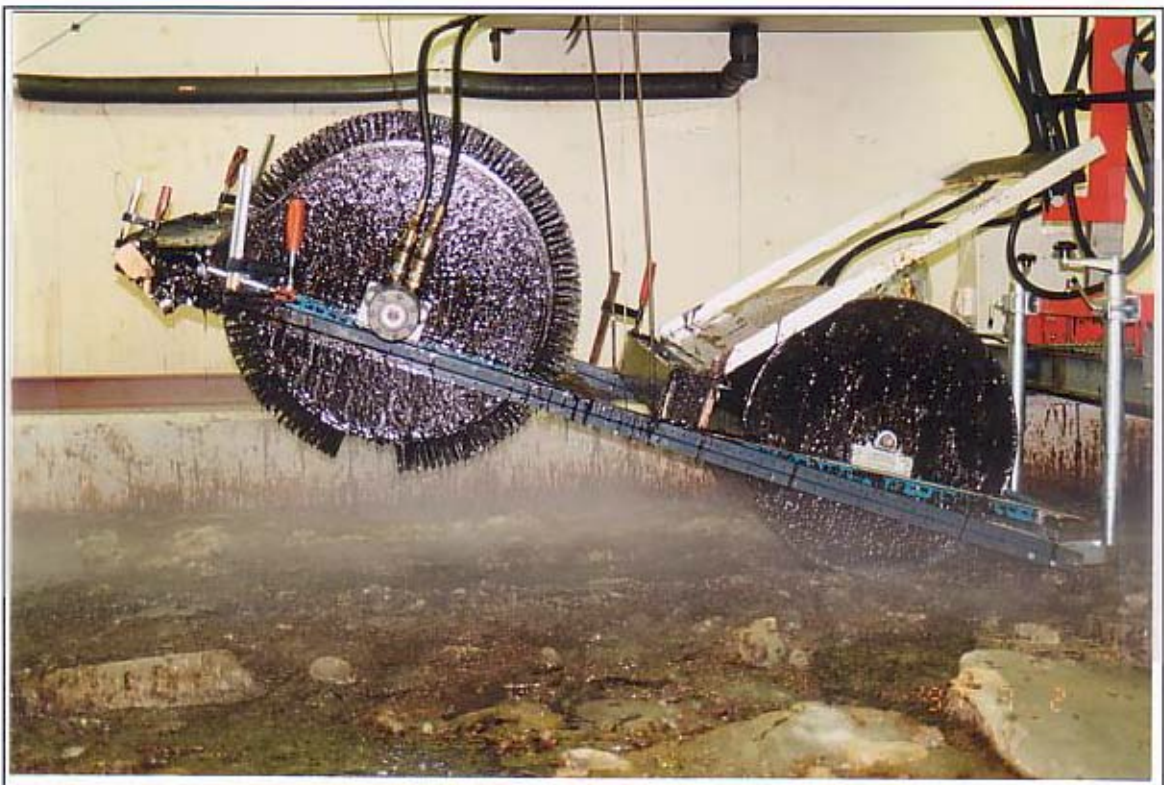
The units were then operated in the opposite direction to study the effects of leading with the spiked drum. Ice no longer accumulated between the units.
