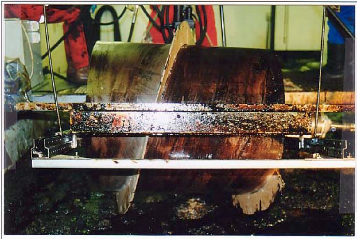
Auger Drum with the longer vane prepared for testing in oil-in-ice conditions.
