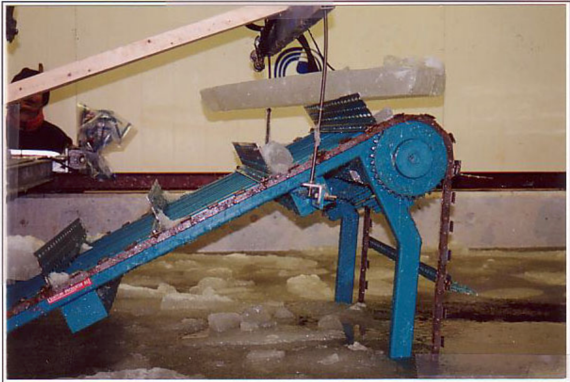
Lifting Grated Belt with first generation paddles which created an upwelling at the front end of the unit, pushing oil and ice away. Seen here deflecting ice over unit.
