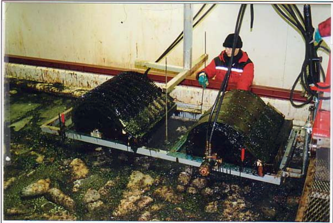
Double Drum testing with the Ringed Brush Drum leading and the Spiked Drum following behind. This configuration resulted in an excessive accumulation of slush and ice pieces between the two drums.
