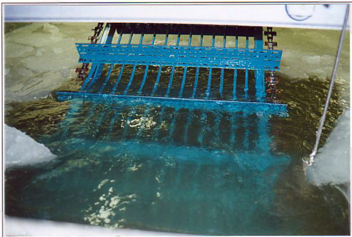
Lifting Grated Belt -first generation lifting paddles create a significant upwelling which drives oil and ice away from unit .
