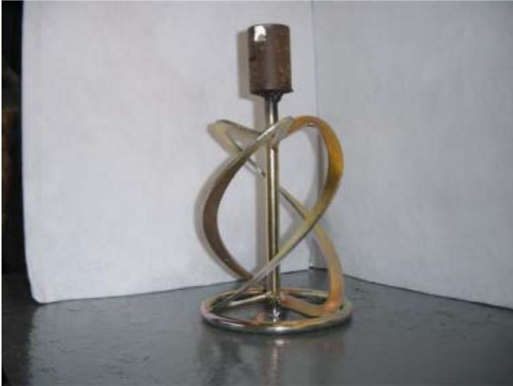
Figure 2 Mechanical Stirrer Used to Make Water-in-Oil Emulsions
