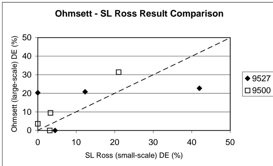
Figure 5 Comparison of Ohmsett (large-scale) and SL Ross (small-scale) DE Results
