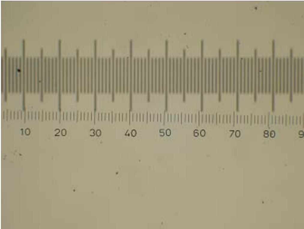
Photo of 1mm/100 Division Stage Micrometer with Eyepiece Reticle Installed (sharper, numbered scale) (60 units on eyepiece reticle = 585 microns on Stage Micrometer or 1 unit = 9.75 microns)
