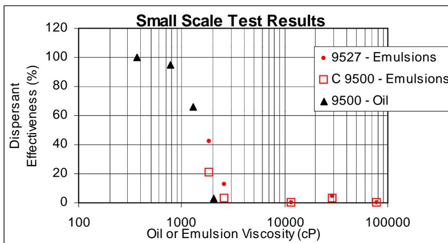
Figure 1 Small-Scale Tank Test Dispersant Effectiveness versus Oil Viscosity
