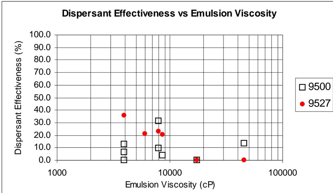
Figure 4 Dispersant Effectiveness vs Emulsion Viscosity in Ohmsett Tank Tests
