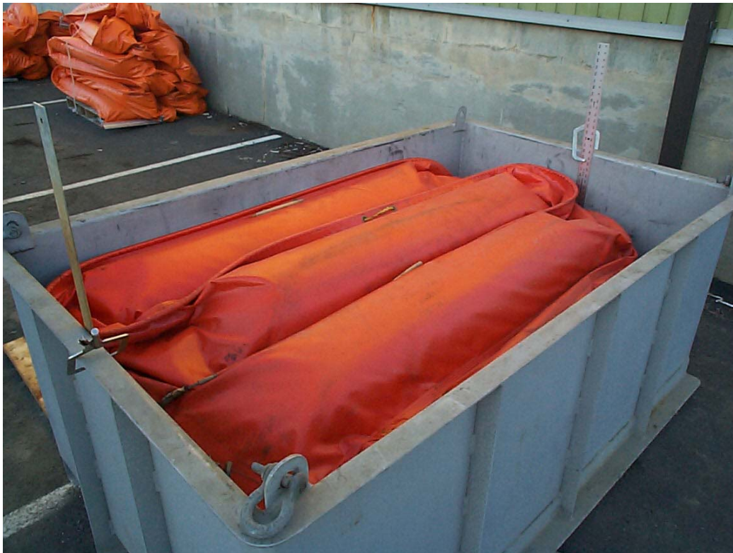
Figure 4: Tank used for measuring boom displacement
