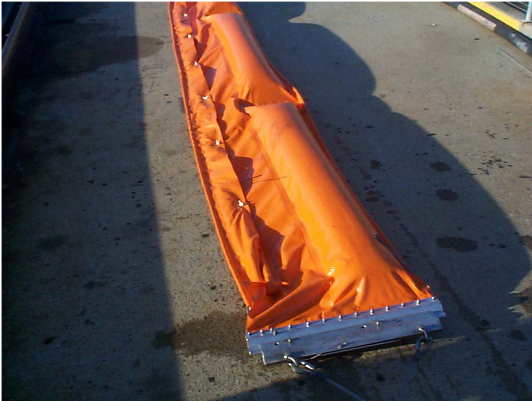
Figure 3: Curtain boom showing chain pocket along bottom edge
