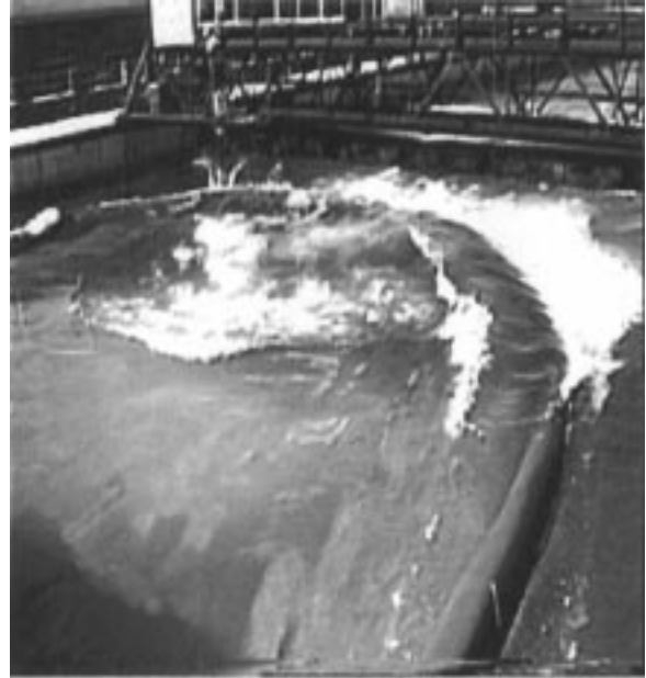
FIG. 5 Critical Tow Speed in Calm Water
