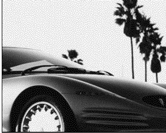
Figure 1. An example of a digital halftone image generated with the direct-binary-search algorithm taken from Ref. 9, which shows the high quality that is achievable with state-of-the-art halftone rendering of gray-scale images. (©IEEE)
