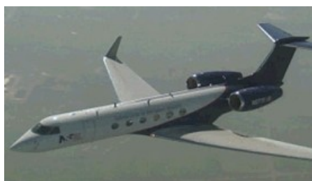
HIAPER, the nation's most advanced research aircraft, just completed its first experiment. A modified Gulfstream V jet, the aircraft can fly at higher altitudes for extended periods and can carry 5,600 pounds of sensing equipment, making it the premier plane for scientific discovery. Credit: NSF.
