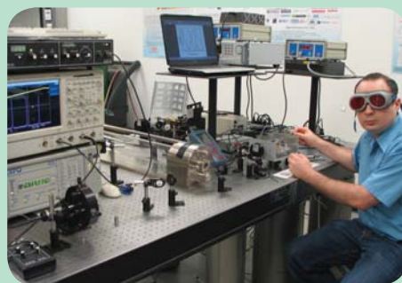
A team of researchers at the University of Alabama at Birmingham, led by physics professor Sergey Mirov, developed a novel laser-based “optical nose” for the rapid identification and quantification of organic trace-gases in multi-compound gas mixtures with full biochemical specificity and high sensitivity. Above, Dmitri Martyshkin uses the optical nose for sensing hydrogen fluoride molecules. Credit: Courtesy Sergey Mirov, University of Alabama at Birmingham
