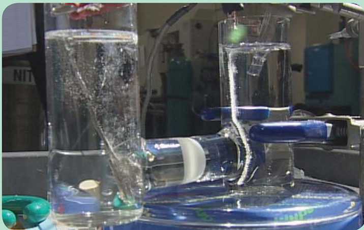
Massachusetts Institute of Technology chemist Daniel Nocera and his postdoctoral student Matthew Kanan discovered this new, efficient catalyst that produces oxygen gas from water. Nocera is a member of Powering the Planet, one of NSF's Centers for Chemical Innovation (CCI). Credit: MIT/NSF
