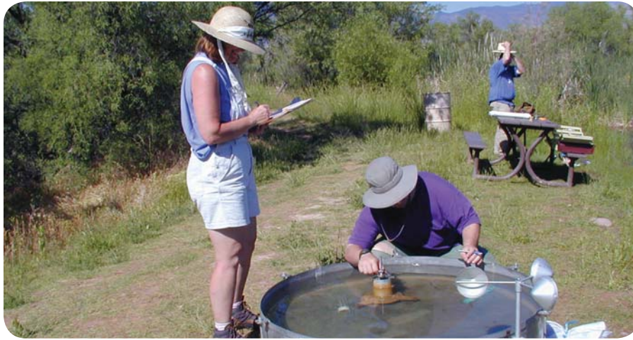
Students measure evaporation rates in Patagonia, Ariz. Data collection is a vital part of the work of the Center for Sustainability of Semi-Arid Hydrology and Riparian Areas (SAHRA), an NSF Science and Technology Center. Credit: Jonathan Pefti, SAHRA, University of Arizona, Tucson
