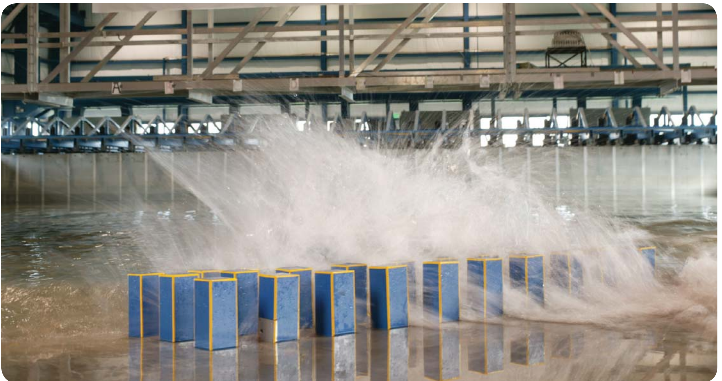
The Tsunami Wave Basin at Oregon State University is the world's largest facility for investigating the effects of large waves. By studying the impact of tsunamis on model buildings (the boxes, above) and other structures, engineers and scientists can develop better designs and materials to mitigate damage to people and property. The Tsunami Wave Basin is part of the George E. Brown, Jr. Network for Earthquake Engineering Simulation (NEES). Credit: College of Engineering, Oregon State University
