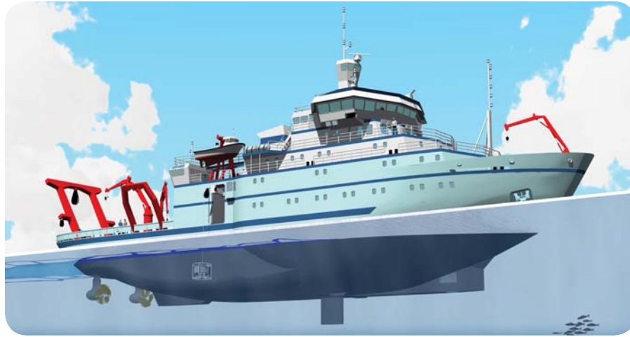
The proposed Alaska Region Research Vessel (ARRV) is designed to operate up to 300 days per year in the harsh, icy waters around Alaska. The ship would provide a much needed platform for addressing critical regional and global ecosystem issues including ocean circulation and climate change. Credit: The Glosten Associates, Inc.
