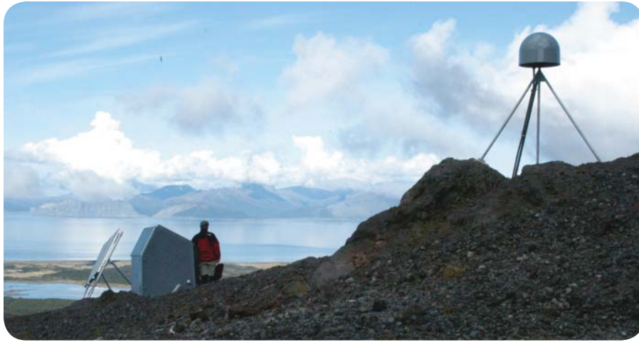
A researcher checks out a Global Positioning System (GPS) station in the Aleutian Islands. EarthScope's Plate Boundary Observatory (PBO) uses an array of permanent, continuously recording GPS stations and strainmeters installed across the North American continent to monitor Earth motion. Credit: EarthScope
