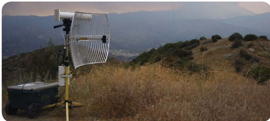
With relays like this one on Palomar Mountain, the High-Performance Wireless Research and Education Network (HPWREN) brought connectivity to firefighters at the scene of the 2003 Coyote wildfire, allowing them to receive weather notices and submit incident summaries in real-time. Before it was brought under control, the fire burned more than 17,000 acres in southern California. Credit: High Performance Wireless Research and Education Network (HPWREN)
