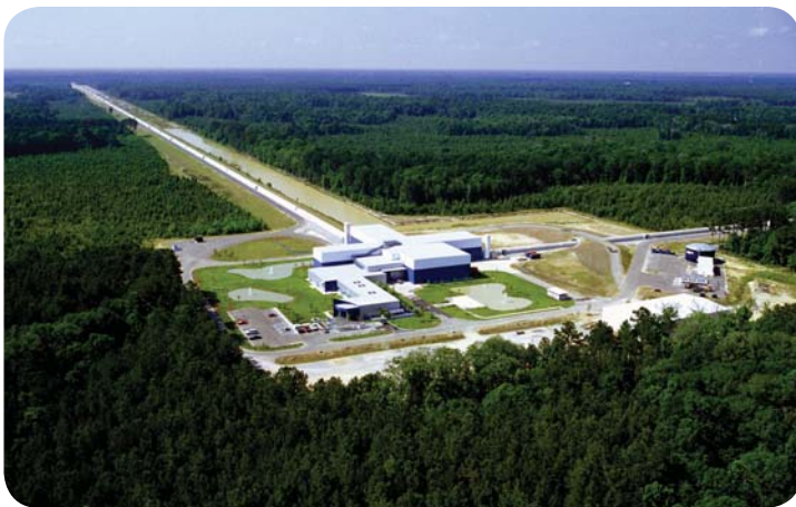
Aerial view of the Laser Interferometer Gravitational-Wave Observatory (LIGO) site at Livingston, La., looking south along one of its two interferometer arms. LIGO consists of three interferometers at two locations—the other location is Hanford, Wash.—that are approximately 3,000 kilometers apart. Credit: LIGO Laboratory, California Institute of Technology
