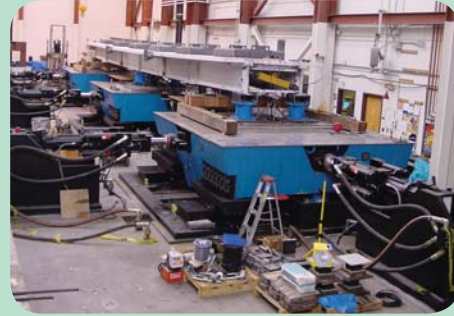
Researchers using the multiple shake table facility at the University of Nevada, Reno—part of the George E. Brown, Jr. Network for Earthquake Engineering Simulation (NEES)—are investigating the performance of large-scale models of four-span bridges and full-scale bridge components. Credit: Lyle Carden, University of Nevada, Reno
