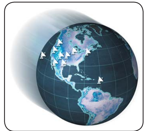
This map shows the locations of the 10 radio antennas of the Very Long Baseline Array (VLBA). The antennas function together as one instrument with very high resolution and sensitivity. Credit: NRAO/AUI
