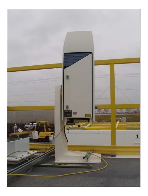
The Ceilometer measures the distance from the ground to the bottom of a cloud directly overhead. This distance is called "cloud base height." The Ceilometer can measure cloud bases up to about 8 kilometers (km) above the surface. The Ceilometer sends out a pulse (flash) of light and measures how long it takes for the light to come back after being reflected off the bottom of a cloud.
