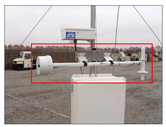
The temperature and humidity sensors are mounted inside a tube to protect them from direct sunlight. The tube is attached to the Meteorological Tower near the bottom. A small fan at one end draws air into the tube and over the sensors.
