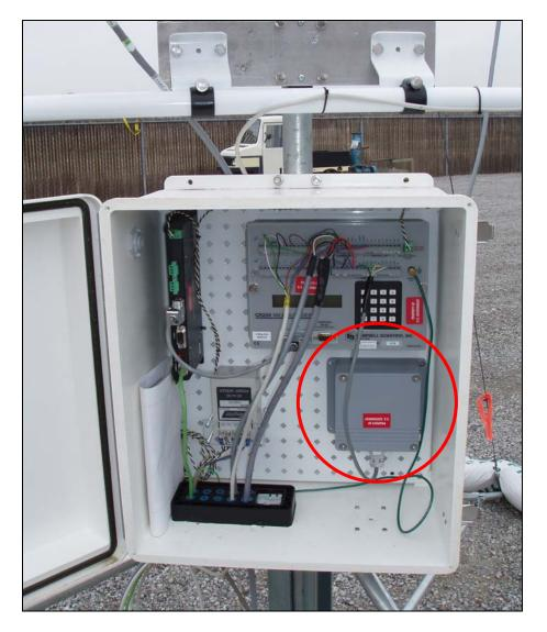
A barometer measures atmospheric pressure and is housed inside the logger container on the Meteorological Tower. A tube connects the barometer to the outside.
