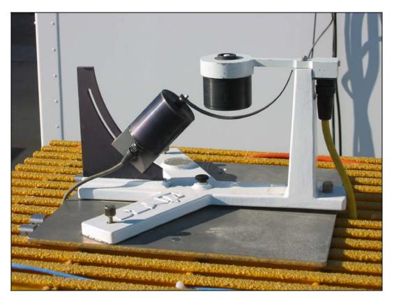
The MFRSR uses measurements of the total and diffuse solar radiation to determine properties of the atmosphere. The MFRSR has a black shading arm that rotates over the sensor every 15 seconds. When the sensor is unshaded, it measures total solar irradiance. When the shading arm blocks the sun from the sensor, the MFRSR measures the diffuse solar irradiance. The direct solar irradiance can be calculated by subtracting the diffuse value from the total value.
