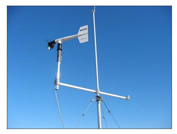
The wind sensor is mounted on the top of the Meteorological Tower. The propeller measures wind speed. The direction of the wind is measured by the position of the vane.
