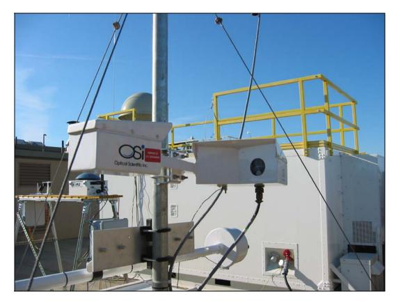
Mounted on the Meteorological Tower, the ORG measures the rate of rainfall in millimeters per hour (mm/hr). It sends an invisible beam of light from one of its ends to a detector at the other end. When raindrops fall, they break the beam. The rain rate is determined by measuring how often the beam is broken. It can be used to calculate the total amount of rain that has fallen in any given period.
