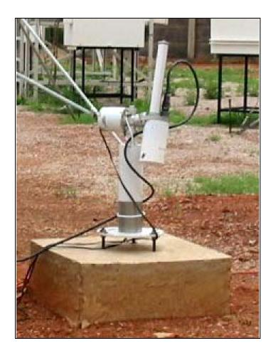
The Cimel Sunphotometer (CIMEL) is a multi-filter, automatic, sun-tracking radiometer that measures aerosol, water vapor, and ozon, as well as the direct solar radiance and reflected sky radiance at the Earth's surface. Measurements are taken at pre-determined discrete wavelengths in the visible and near-infrared parts of the spectrum to determine atmospheric transmission and scattering properties. The CIMEL operates only during daylight hours (i.e., sun above horizon).
