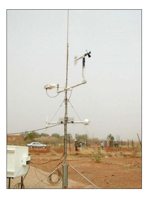
Propeller Vane Wind Sensors (WND)
