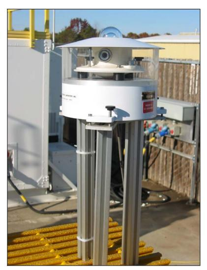
The PSP measures the amount of solar radiation (sunshine) that falls on the sensor under the clear dome. When pointed upward unshaded, the PSP measures the total amount of solar radiation coming directly from the sun plus the radiation that is scattered downwards by clouds, other material in the air, and the air itself. This value is called the "total" or "global" solar irradiance. The value is reduced when clouds are present.
