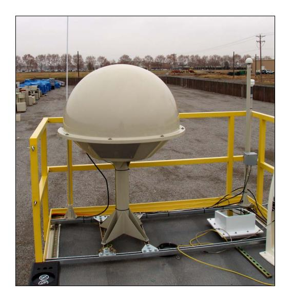
The Balloon-Borne Sounding System provides vertical profiles of both the thermodynamic state (i.e., temperature) of the atmosphere and the wind speed and direction. The data are collected by a radiosonde attached to a weather balloon. The main components of the BBSS are a radiosonde, a balloon, an antenna to receive data (shown above), and DigiCORA, a computer program that collects data from the radiosonde.
