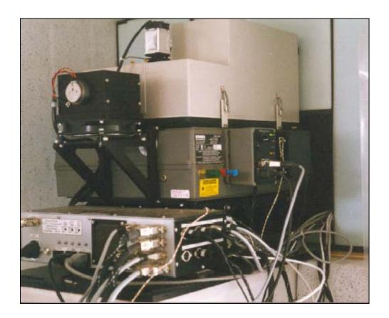
The AERI measures a spectrum of heat radiation of the sky directly above the instrument. A spectrum is a distribution of energy across a range of wavelengths. Because the AERI measures a spectrum of heat radiation, its data produce profiles of temperature and water vapor of the atmosphere above the instrument. Scientists also use the AERI data to improve models of how heat radiation behaves in the Earth's atmosphere.
