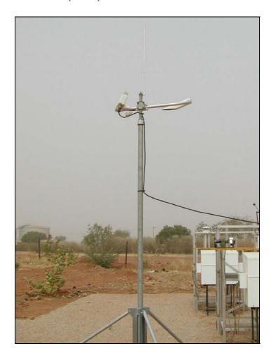
The Present weather Detector (PWD) measures the visibility near the surface by estimating the water content of precipitation and combining it with optical forward scatter and temperature measurements. The AMF is equipped with the Vaisala PWD22, which measures visibility up to 20 km depending on the weather condition.
