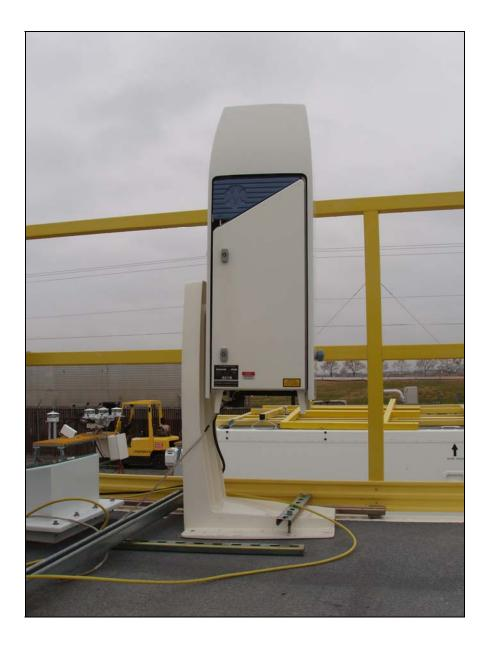
The Ceilometer measures the distance from the ground to the bottom of a cloud directly overhead. This distance is called "cloud base height." The Ceilometer can measure cloud bases up to about 8 kilometers (km) above the surface. The Ceilometer sends out a pulse (flash) of light and measures how long it takes for the light to come back after being reflected off the bottom of a cloud.
