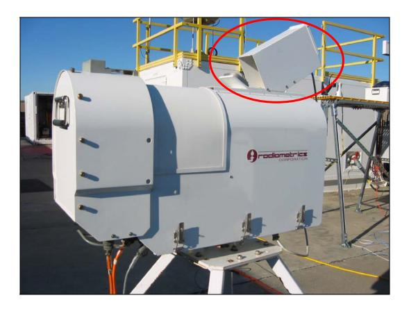
The MWRP provides continuous profiles of water vapor, liquid water, and temperature up to 10 km height. Those profiles are obtained at 10-second intervals during clear, cloudy, and precipitating conditions. The temperature measurements are taken with the Infrared Thermometer (IRT) mounted on top.
