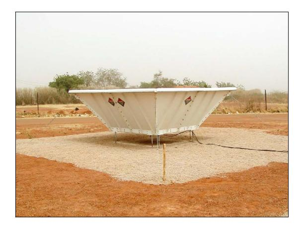
The RWP measures wind profiles from 2 to 5 km and virtual temperature profiles from 1 to 2 km by transmitting electromagnetic energy into the atmosphere and measuring the strength and frequency of backscattered energy.
