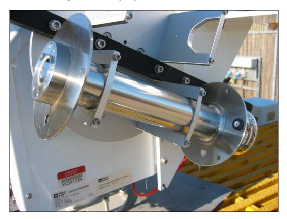
The NIP is like a narrow view telescope. It has a sensor at the viewing end that measures the amount of solar radiation that falls on it. The NIP is mounted on the solar tracker so that it is always pointing directly at the sun. The value is called the "direct" solar irradiance. This value decreases when the sun is lower in the sky. When thick clouds are present (that is when the solar disk cannot be seen), the NIP should measure approximately zero.
