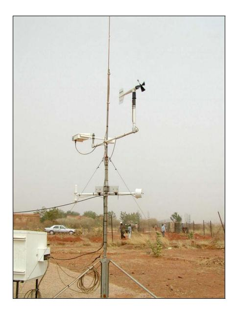
**Propeller Vane Wind Sensors (WND)**
