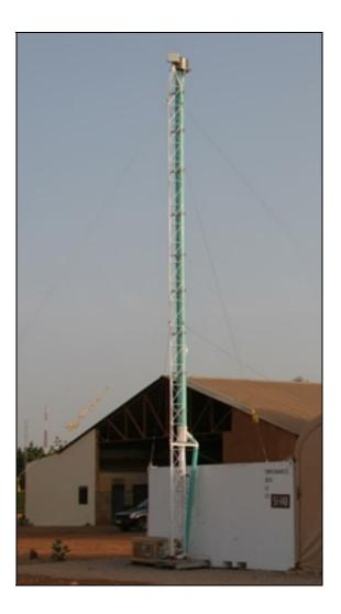
The AOS takes in-situ aerosol measurements at the surface. The principal measurements are the aerosol absorption and scattering coefficients as a function of the particle size and radiation wavelength. Additional measurements include the particle number concentration, size distribution, hygroscopic growth, and inorganic chemical composition. The AOS measures aerosol optical properties to better understand how particles interact with solar radiation and influence the earth's radiation balance.
