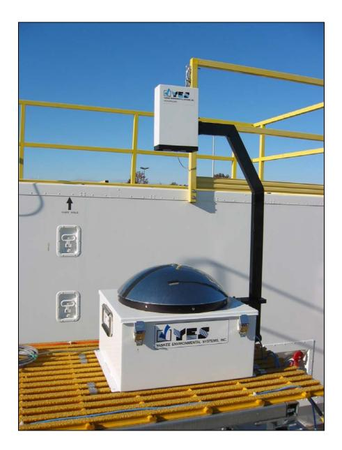
The Total Sky Imager (TSI) provides time series of hemispheric sky images during daylight hours, and retrievals of fractional sky cover for periods when the solar elevation is greater than 5 to 10 degrees.
