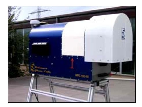
The Microwave Radiometer - High Frequency (MWRHF) provides time-series measurements of brightness temperatures from two channels centered at 90 and 150 GHz. These two channels are sensitive to the presence of liquid water and precipitable water vapor.
