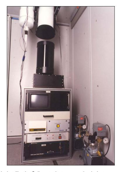
The MPL works just like the Ceilometer but can see clouds that are much higher. The MPL can detect cirrus clouds, which can be as high as 16 to 17 km high.
