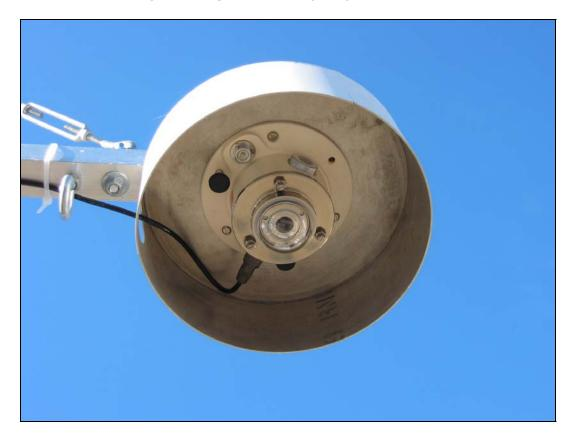
The PSP measures the amount of solar radiation (sunshine) that falls on the sensor under the clear dome. When the PSP is pointed downward, it measures the amount of solar radiation reflected from the surface below. The value depends on the amount of sunshine hitting the surface and how well the underlying surface reflects the sunshine.
