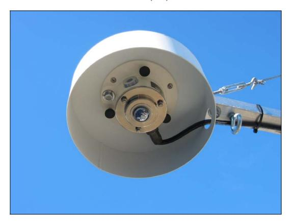
The PIR measures the amount of infrared (heat) energy that falls on a sensor under the shiny dome. This energy is the same heat energy you feel when standing next to a campfire or cook stove. The shiny dome reflects solar radiation but allows infrared radiation to pass through. When the PIR is pointed downward, it measures the upwelling infrared irradiance or heat energy given off by the surface below.
