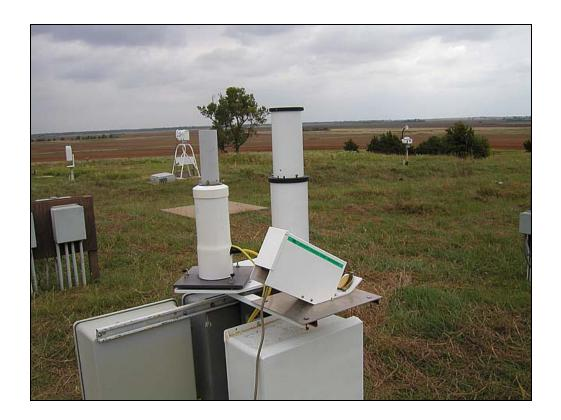
The 2-Channel Narrow Field of View Zenith Radiometer (2NFOV) is a ground-based radiometer that looks straight up in the sky. With its narrow field of view, the 2NFOV measures the downwelling zenith radiance in a 1-second time series. The radiance is measured at a wavelength of 869 nm. One example of the uses for the data collected by this instrument is to examine the internal structure of clouds.
