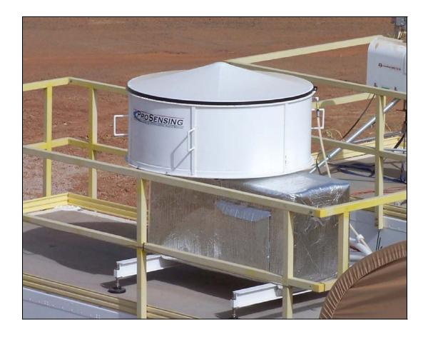
The W-band ARM Cloud Radar is a zenith-pointing radar that operates at a frequency of 95 GHz. The main purpose of this radar is to determine cloud boundaries (i.e., cloud bottoms and tops). This radar can also report radar reflectivity (dBZ) of the atmosphere up to 20 km. In addition, the WACR has a Doppler capability that allows the measurement of cloud constituent vertical velocities.
