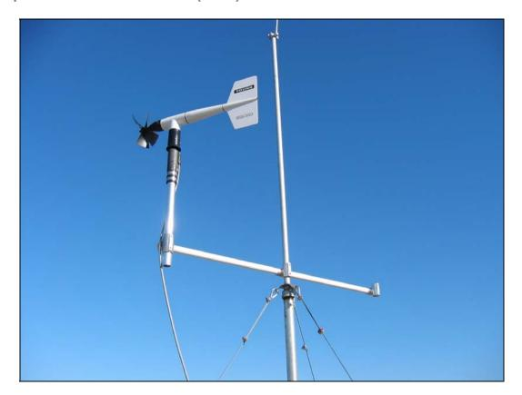
The wind sensor is mounted on the top of the Meteorological Tower. The propeller measures wind speed. The direction of the wind is measured by the position of the vane.
