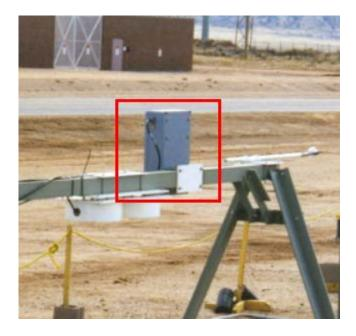
The IRT measures the temperature of an object that it is pointing at by measuring the infrared radiation coming from the object. If you pointed it at a cooking fire it would tell you the temperature of the fire.
