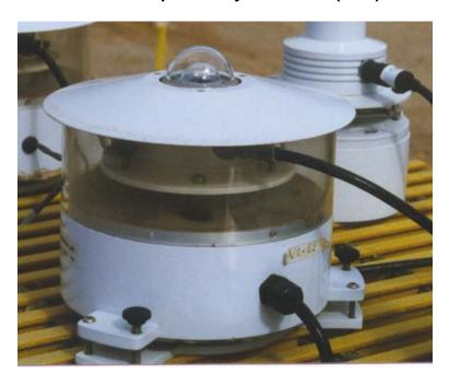
The PSP measures the amount of solar radiation (sunshine) that falls on the sensor under the clear dome.
