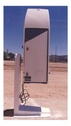
The Ceilometer is located near the back of the instrument van. The Ceilometer measures the distance from the ground to the bottom of a cloud directly overhead. This distance is called "cloud base height." The Ceilometer can measure cloud bases up to about 8 kilometers above the surface. The Ceilometer sends out a pulse (flash) of light and measures how long it takes for it to come back to the Ceilometer after being reflected off the bottom of a cloud.
