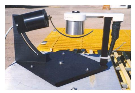
The MFRSR uses measurements of the total and diffuse solar radiation to determine properties of the atmosphere. The MFRSR has a black shading arm that rotates over the sensor every 15 seconds. When the sensor is unshaded it measures total solar irradiance. When the shading arm blocks the sun from the sensor, the MFRSR measures the diffuse solar irradiance. The direct solar irradiance can be calculated by subtracting the diffuse value from the total value.
