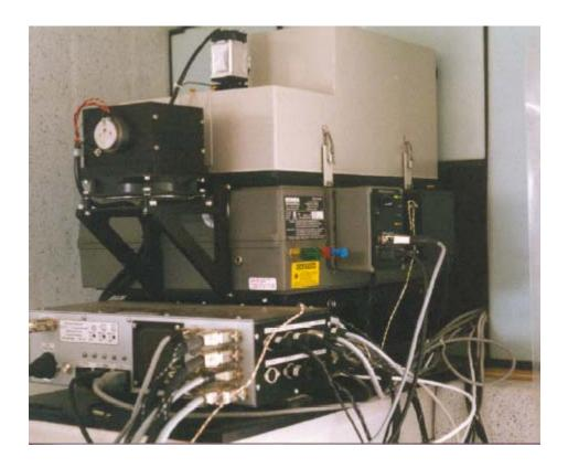
The AERI measures a spectrum of heat radiation of the sky directly above the instrument. A spectrum is a distribution of energy across a range of wavelengths. Because the AERI measures a spectrum of heat radiation, its data produces profiles of temperature and water vapor of the atmosphere above the instrument. Scientists also use the AERI data to improve models of how heat radiation behaves in the earth's atmosphere.
