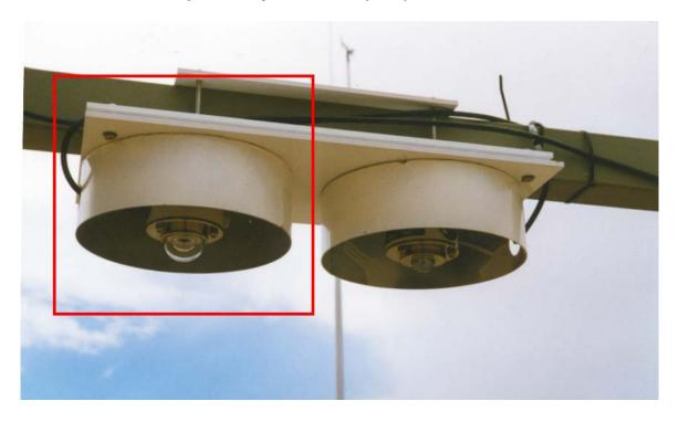
The PSP measures the amount of solar radiation (sunshine) that falls on the sensor under the clear dome.
