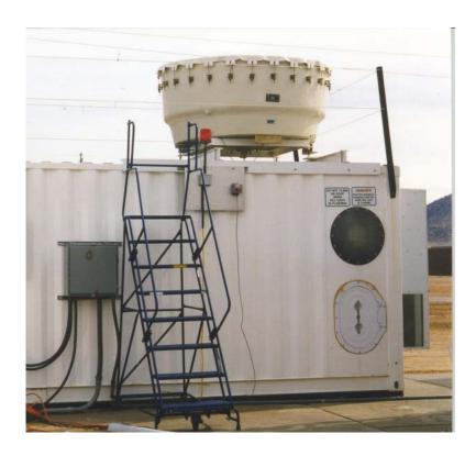
The MMCR is a zenith-pointing radar that operates at a frequency of 35 GHz. The main purpose of this radar is to determine cloud boundaries (e.g., cloud bottoms and tops). This radar will also report radar reflectivity (dBZ) of the atmosphere up to 20 km. The radar has a doppler capability that allows the measurement of cloud constituent vertical velocities.
