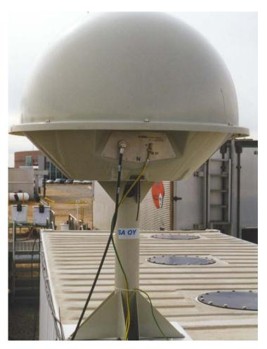
The Balloon-Borne Sounding System (BBSS) provides in situ measurements (vertical profiles) of both the thermodynamic state of the atmosphere and the wind speed and direction.
