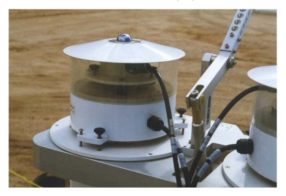
The PIR measures the amount of infrared (heat) energy that falls on a sensor under the shiny dome. This energy is the same heat energy you feel when standing next to a campfire or cook stove. The shiny dome reflects solar radiation but allows infrared radiation to pass through.
