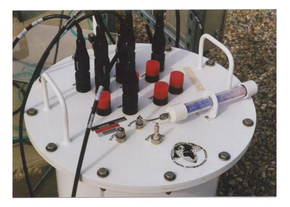
A barometer is housed inside the white cylinder at the base of the meteorological tower. A tube connects the barometer to the outside. Moisture is prevented from entering the barometer by a larger tube filled with water absorbing material. This cylinder also contains a special type of computer (called a datalogger) that collects from the instruments.
