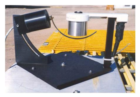
The MFRSR uses measurements of the total and diffuse solar radiation to determine properties of the atmosphere. The MFRSR has a black shading arm that rotates over the sensor every 15 seconds. When the sensor is unshaded it measures total solar irradiance. When the shading arm blocks the sun from the sensor, the MFRSR measures the diffuse solar irradiance. The direct solar irradiance can be calculated by subtracting the diffuse value from the total value.
