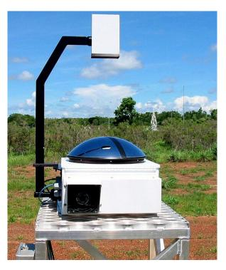
The Total Sky Imager (TSI) provides time series of hemispheric sky images during daylight hours, and retrievals of fractional sky cover for periods when the solar elevation is greater than 5 to 10 degrees.
