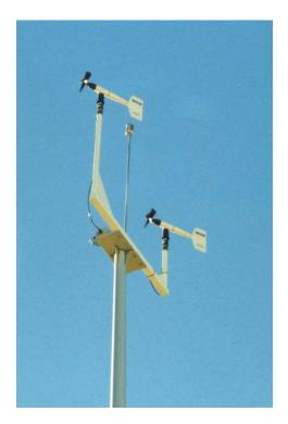
Two propeller vane wind sensors are mounted on the top of the meteorological tower. The propeller measures the wind speed. The direction of the wind is measured by the position of the vane. There are two propeller vanes so that data is not missed if one should fail.
