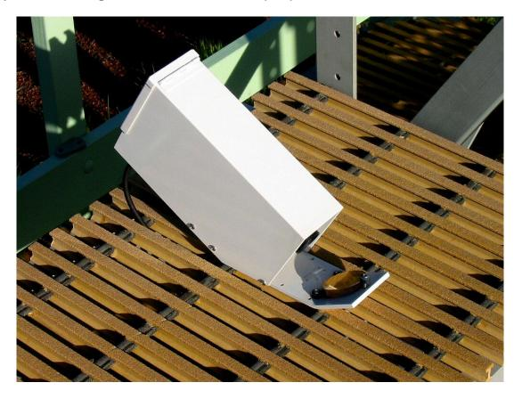
The IRT measures the temperature of an object that it is pointing at by measuring the infrared radiation coming from the object. If you pointed it at a cooking fire it would tell you the temperature of the fire.
