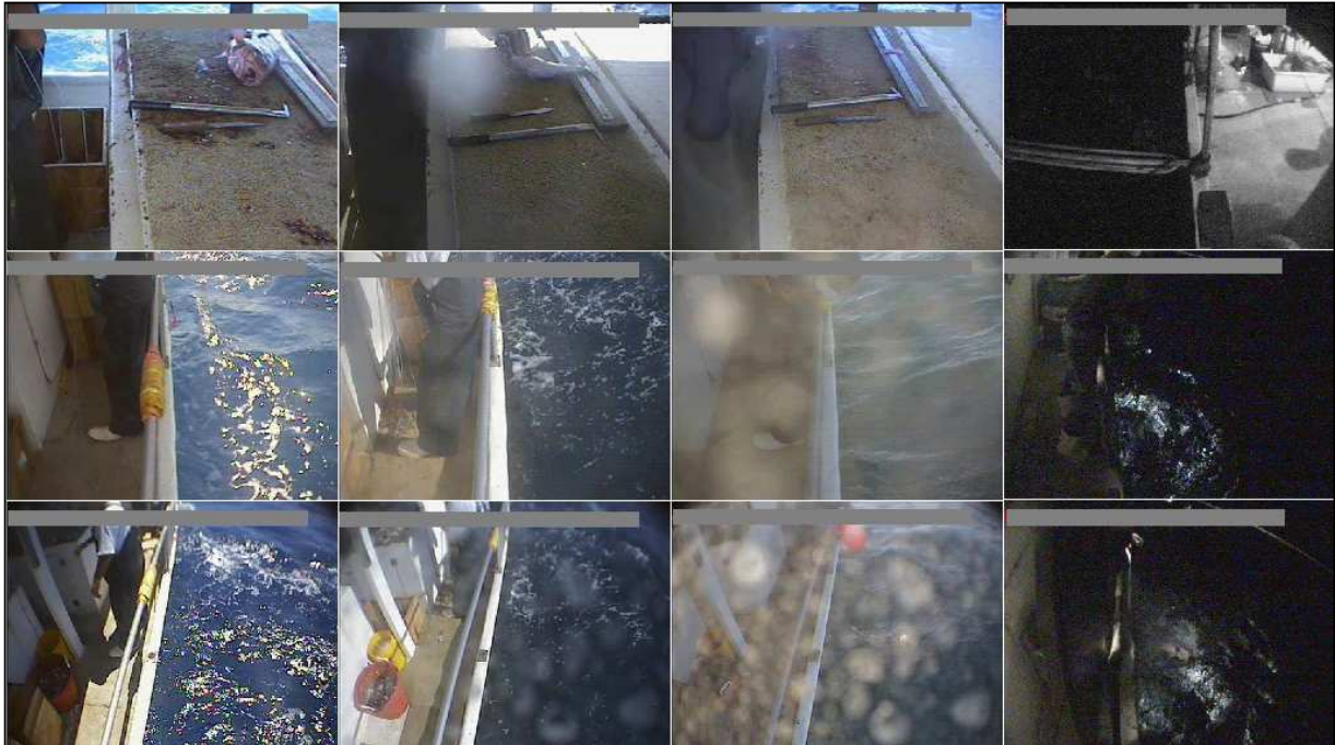
Figure 7. Example imagery to illustrate the different image quality assessments. From left to right: high, medium, low, and unusable. Image quality is determined as an average of all cameras throughout an entire haul. Some cameras may yield a better angle and image clarity than others within the same haul but it is the overall ability to meet imagery review objectives that ultimately determines the imagery quality rating.
