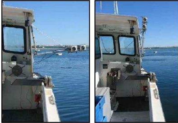
Figure A3 Installation showing a swing arm camera mount.
