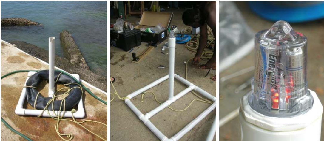
Figure 3. Standardized net marking light stands used to mount Lindgren-Pitman Electralume® white (control) and red (experimental) LED lights.
