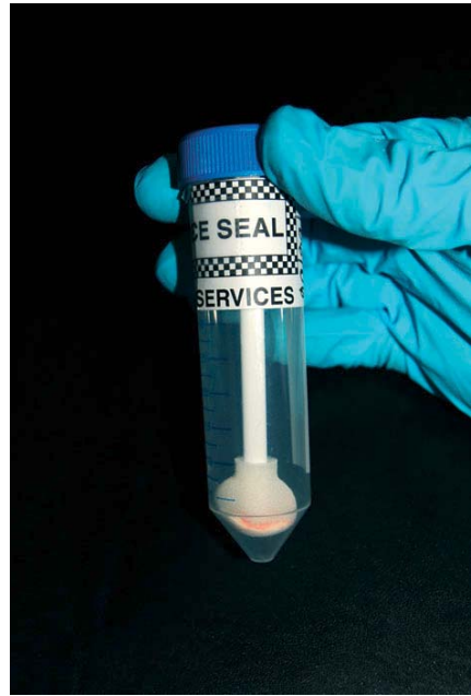
Foam-tip applicator for trace collection.
