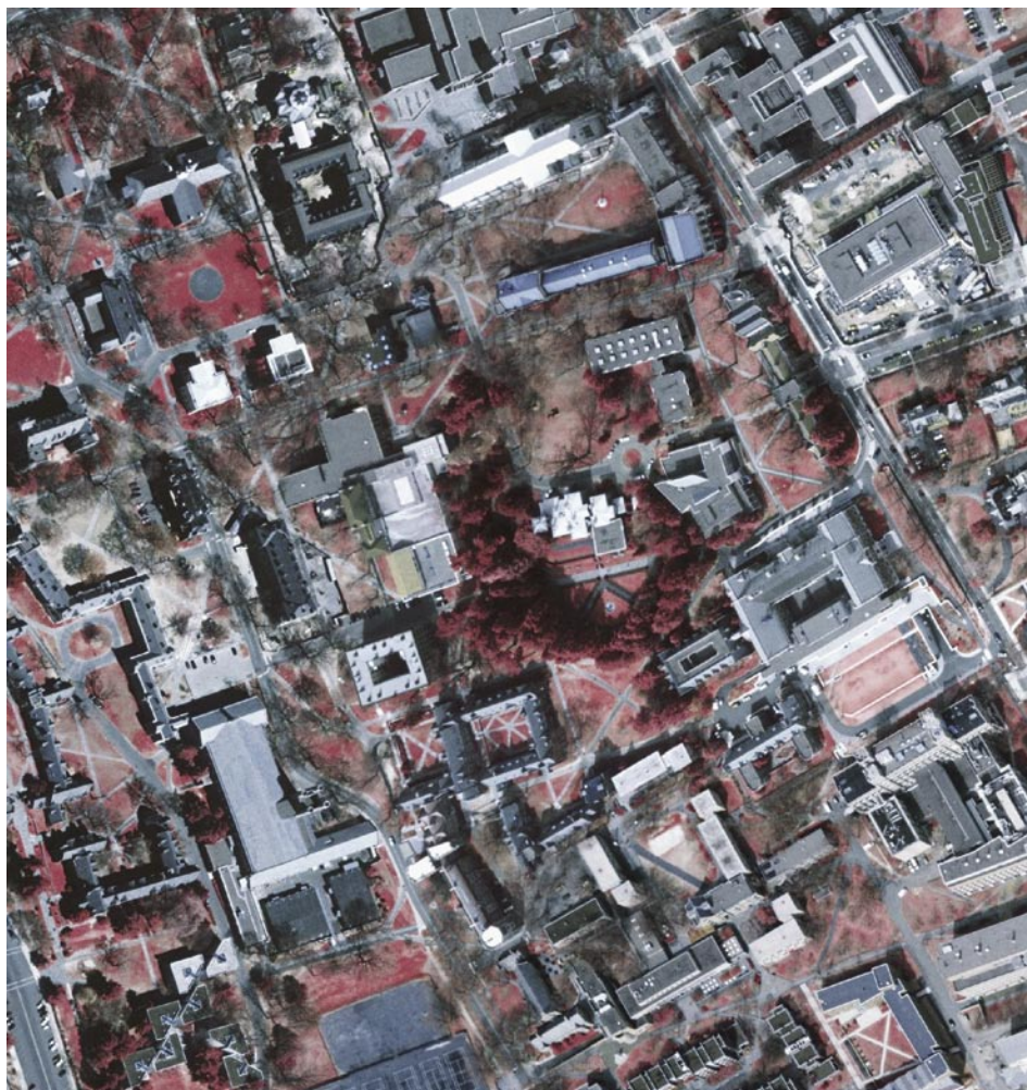
Example of imagery acquired through an agreement with a State. High resolution CIR imagery of a portion of Princeton University acquired through agreement with the State of New Jersey. Pixel resolution is 1 foot.
