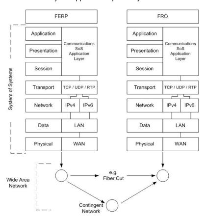
The contingent network in the diagram above is any available WAN connection. If a WAN connection is not available at the incident site, the RPCK will include a small broadband satellite system, with active service.
