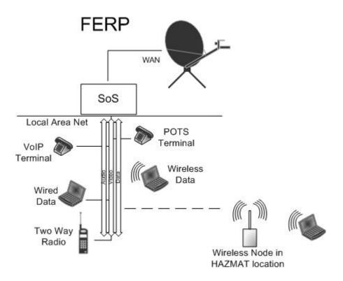
Within 10 to 20 minutes of the FERPs' arrival at the incident area, IACC should be able to move into rescue operations. The system must now move to providing LAN and WAN capability, allowing responding personnel and agencies the ability to interoperate immediately:
