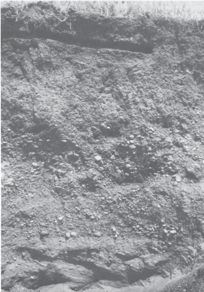
Figure 13.—Profile of Saude loam showing sand and gravel at a depth of about 2 feet.
