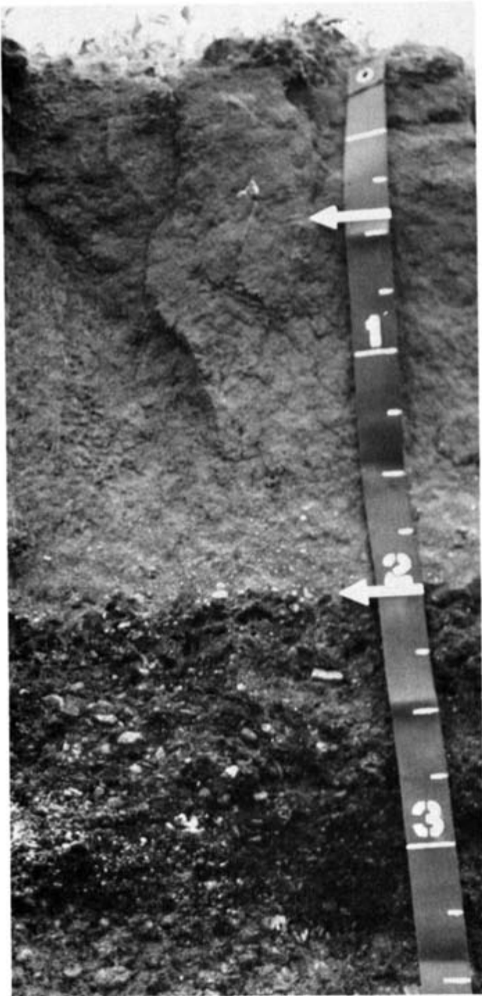
Figure 10.—Profile of Wadena loam, 24 to 32 inches to sand and gravel, 0 to 2 percent slopes. Depth is marked in feet.
