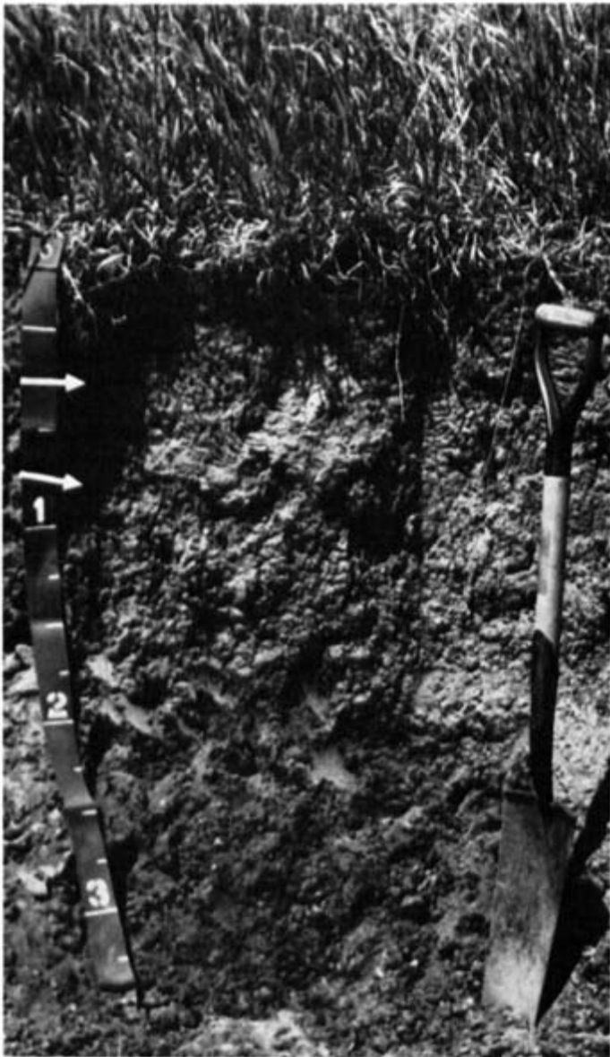
Figure 15.—Profile of Lester loam, 5 to 9 percent slopes. The arrows at depths of 6 and 10 inches indicate the thickness of the subsurface layer. Depth is marked in feet.
