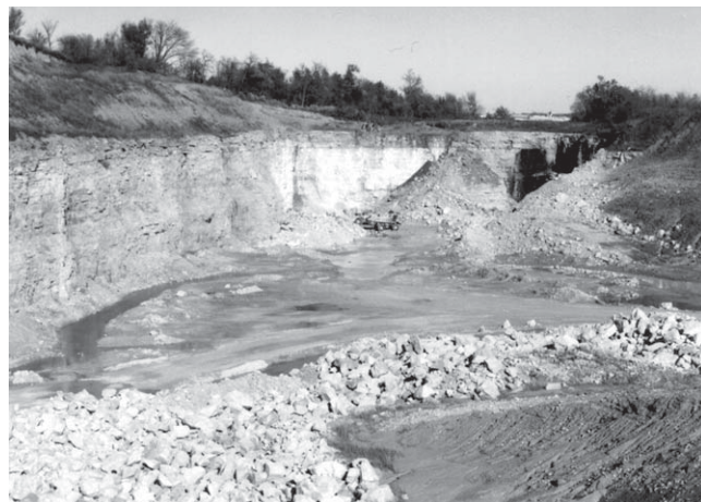
Figure 8.—Mining in an area of Pits, limestone quarries. Limestone is used as an aggregate for cement. Also, applications of limestone in cropped areas can raise the pH of the soils and improve crop growth.
