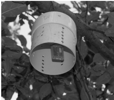
Shelter for keeping the temperature gathering sensor
