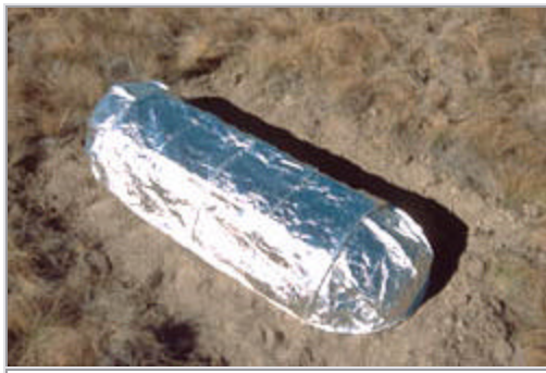
Figure 1 - New fire shelter
